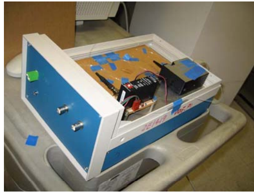
Figure 3.2: The picture of the Ocean-Optics spectrometer-based white-light interferometry system.
