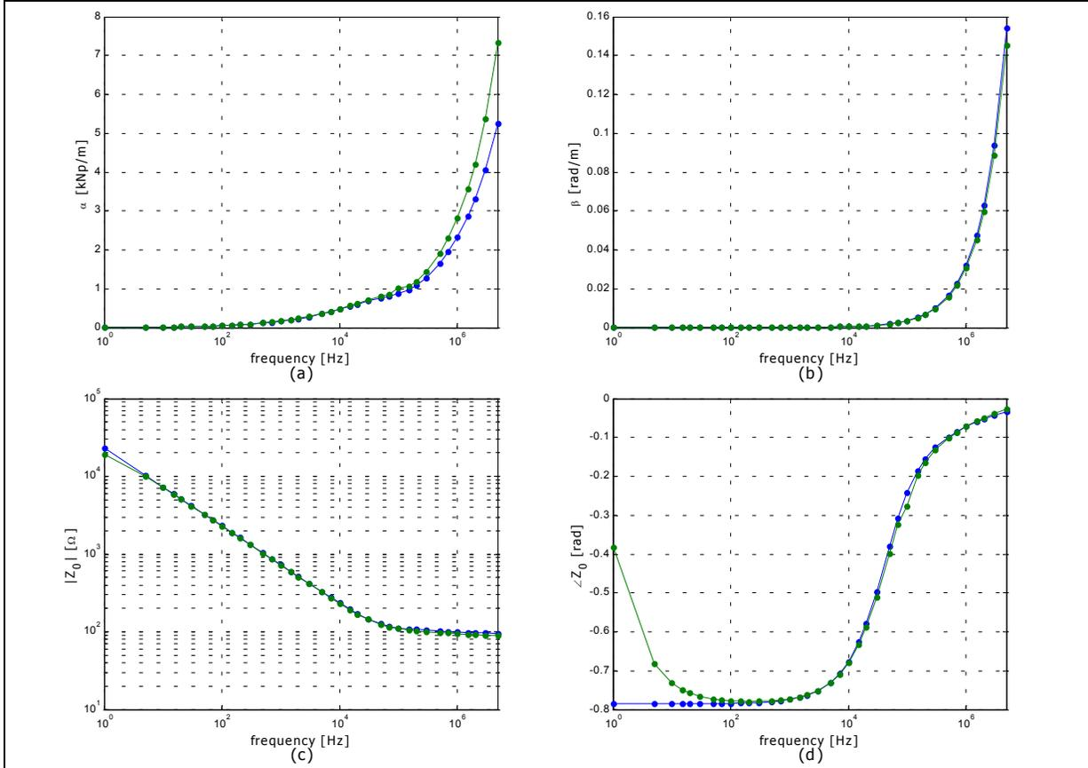
Figure 1-3: PIC (blue), and pulp (green) insulated 24-AWG twisted-pair electrical characteristics – attenuation function (a), phase function (b), magnitude (c) and phase (d) of characteristic impedance.
