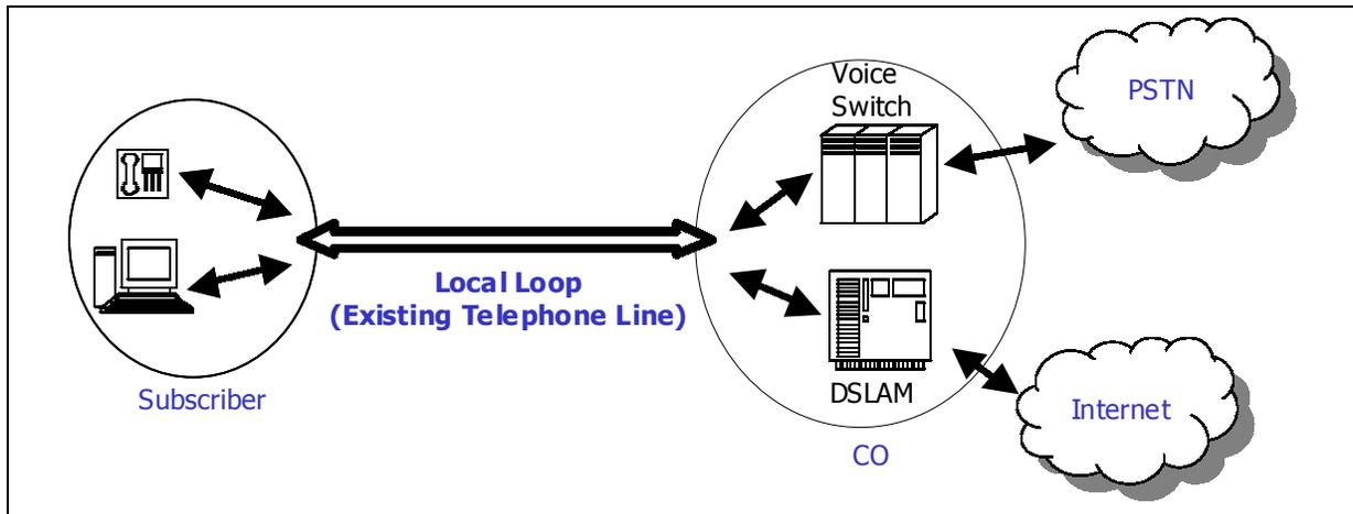
Figure 1-1: Simplified DSL Architecture.
