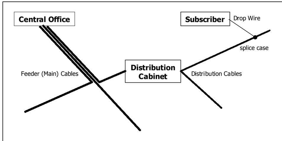
Figure 1-4: General structure of telephone subscriber loop.
