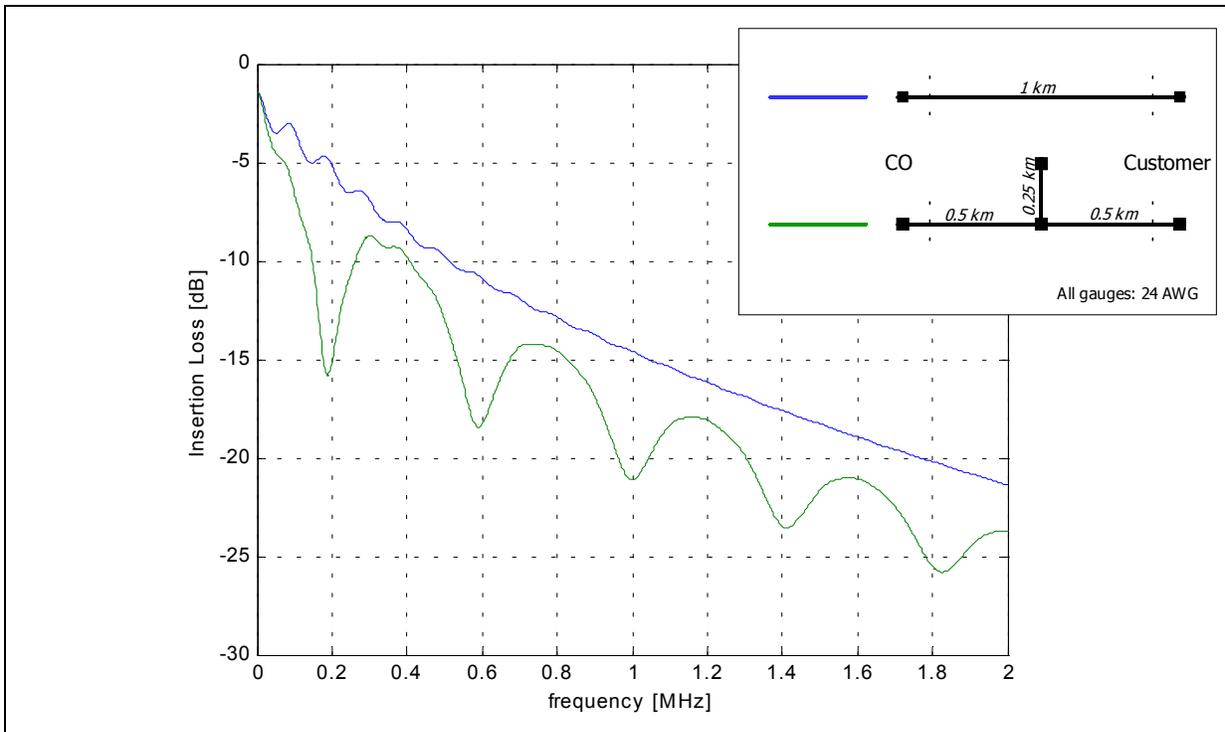
Figure 1-6: Insertion loss due to single 1-km 24-AWG segment loop (blue), and result of adding a 250-m 24-AWG BT to the loop at midway (green).
