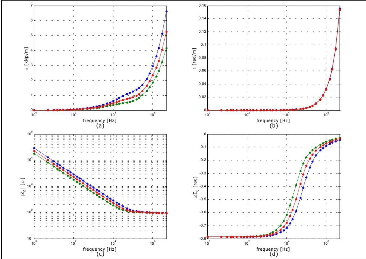
Figure 1-2: Twisted-pair electrical characteristics for 22 AWG (green), 24 AWG (red), and 26 AWG (blue) – attenuation function (a), phase function (b), magnitude (c) and phase (d) of characteristic impedance.
