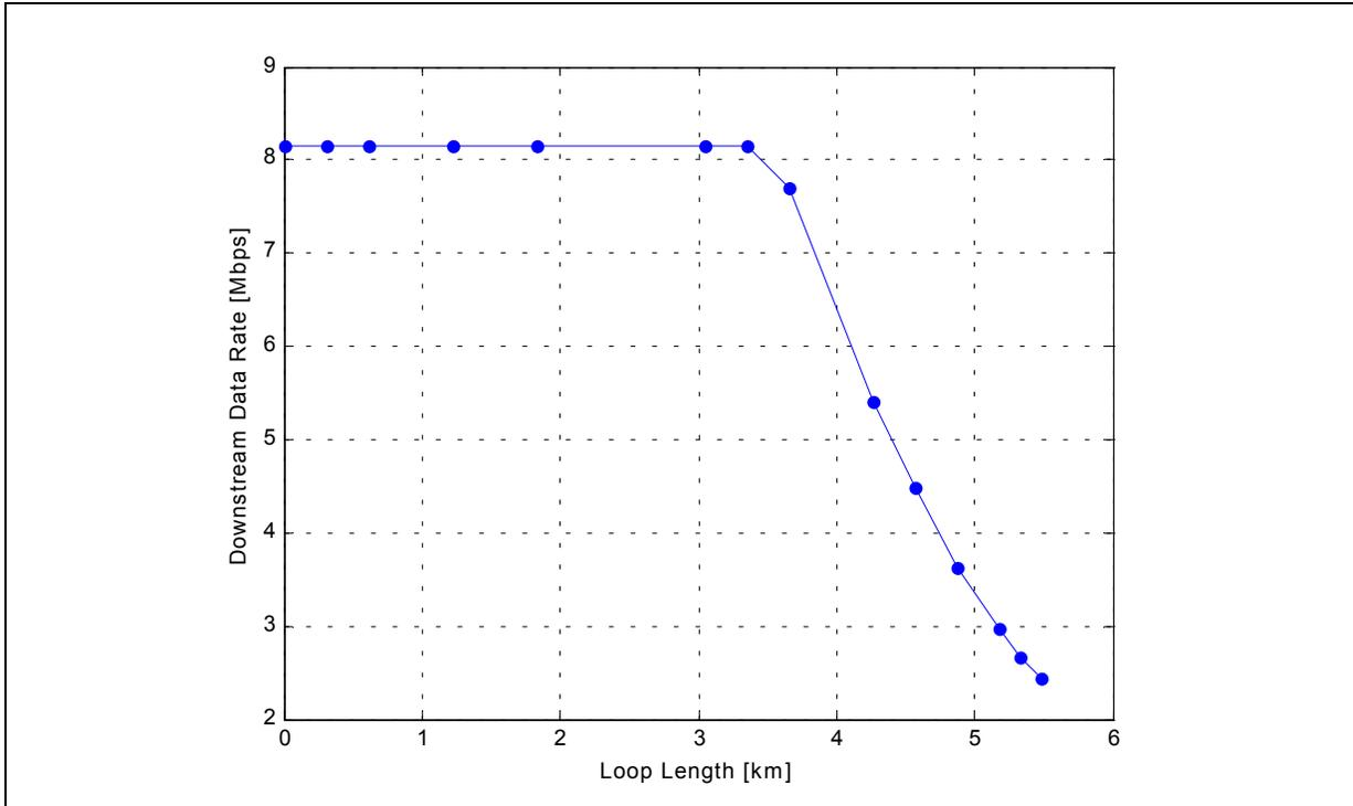
Figure 1-5: Texas Instruments Study — Simulated ADSL downstream data rate as function of length of single 24-AWG segment.
