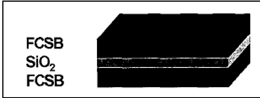
Figure 1.2-6: Sketch of a FeCoBSi double layer with crossed anisotropy [15] (©[2004] IEEE)
