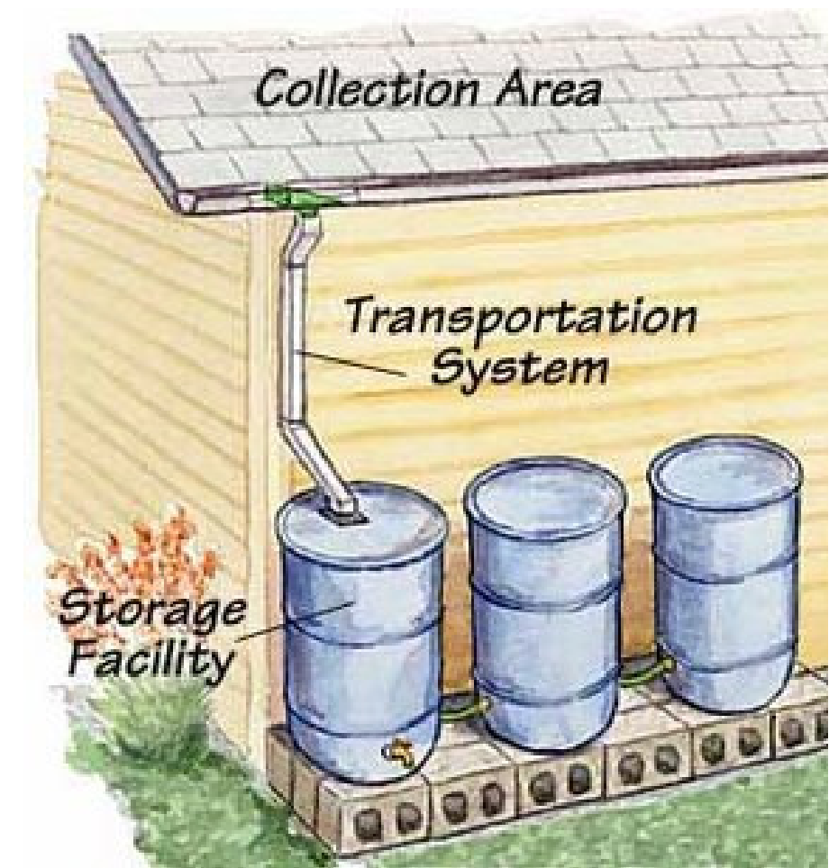
Figure 3.5: Rooftop catchment area (Source: www.lastormwater.info/blog , 2011)
