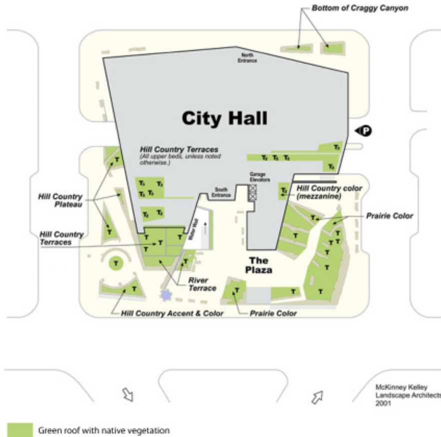
Figure 2.16: Green roof plan of Austin City Hall, Texas (Source: www.eot.state.ma.us/smartgrowth , 2011)
