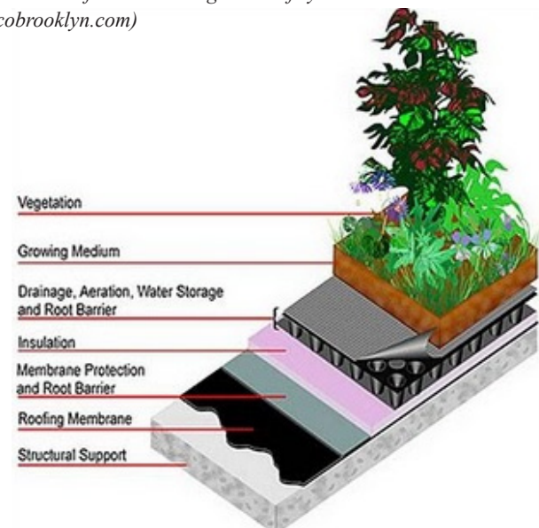
Figure 2.9: Section of an intensive green roof system (Source: www.lowimpactdevelopment.org)
