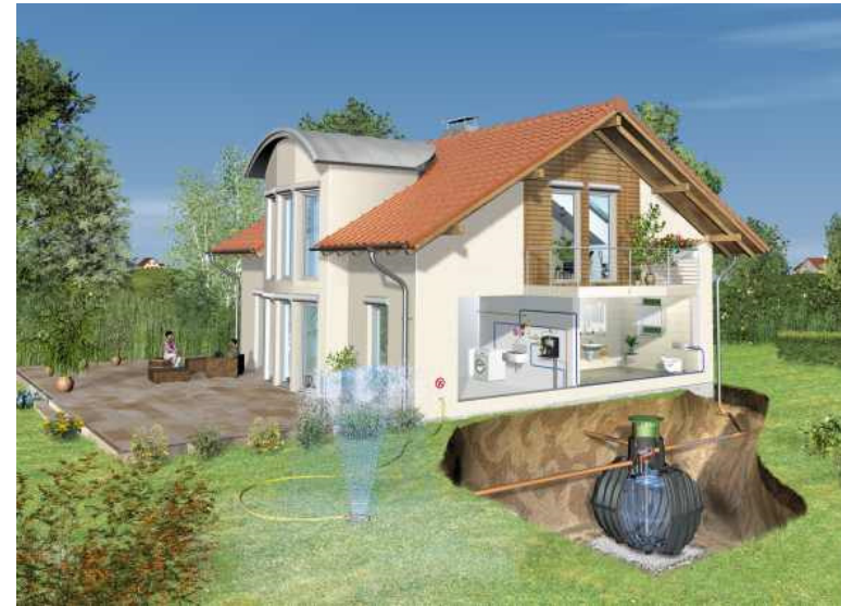
Figure 3.4: Underground Rainwater Harvesting System (Source: www.oak-barrel.com/house_rainwater_supply , 2011)
