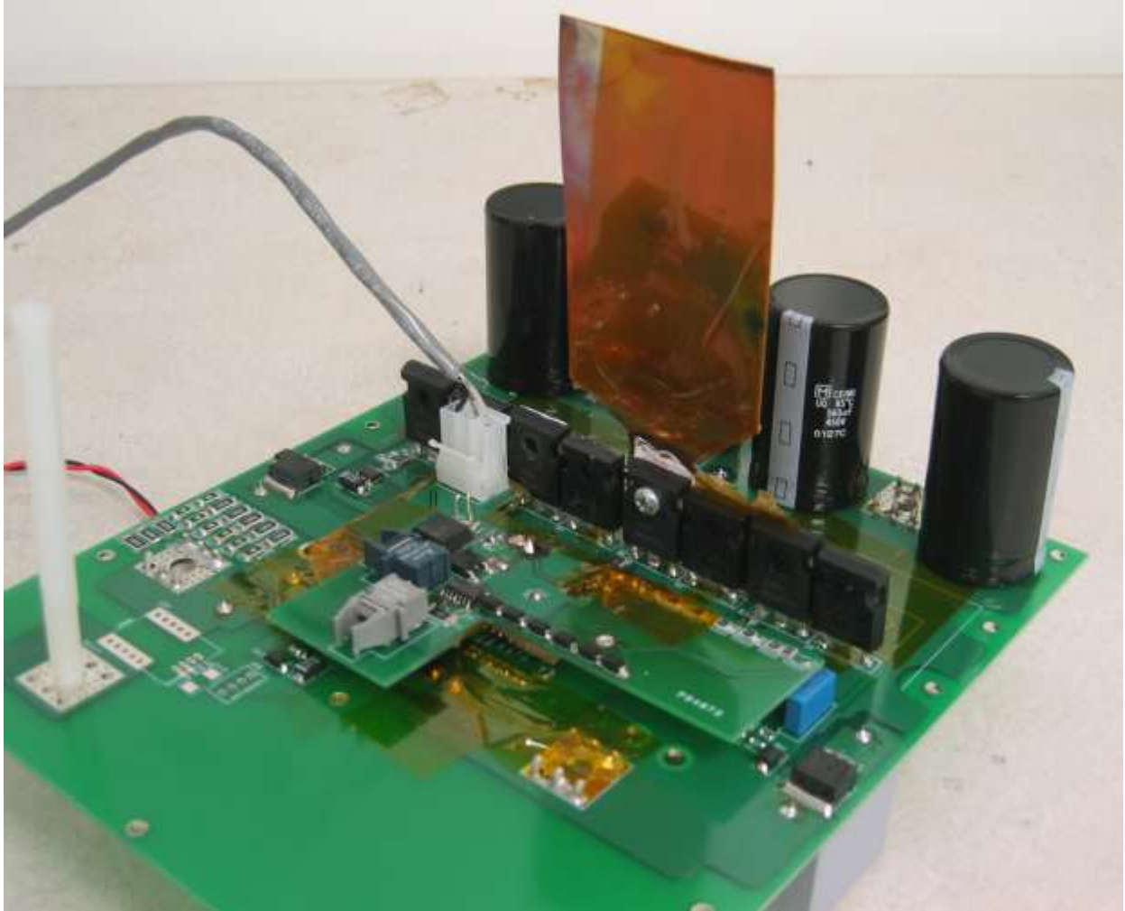
Figure 31: Device driver with CoolMOS, ultra-fast EPU06 diode, four aluminum electrolytic capacitors, and FFB film bypass capacitor (not shown)
