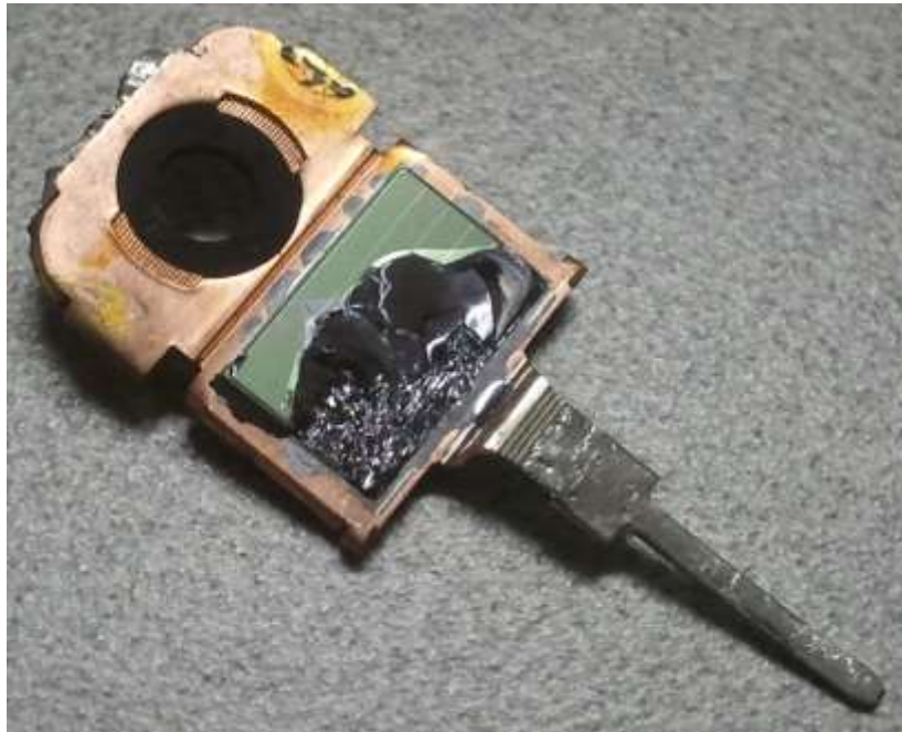
Figure 75: Drain pin attached to tab with damaged die
