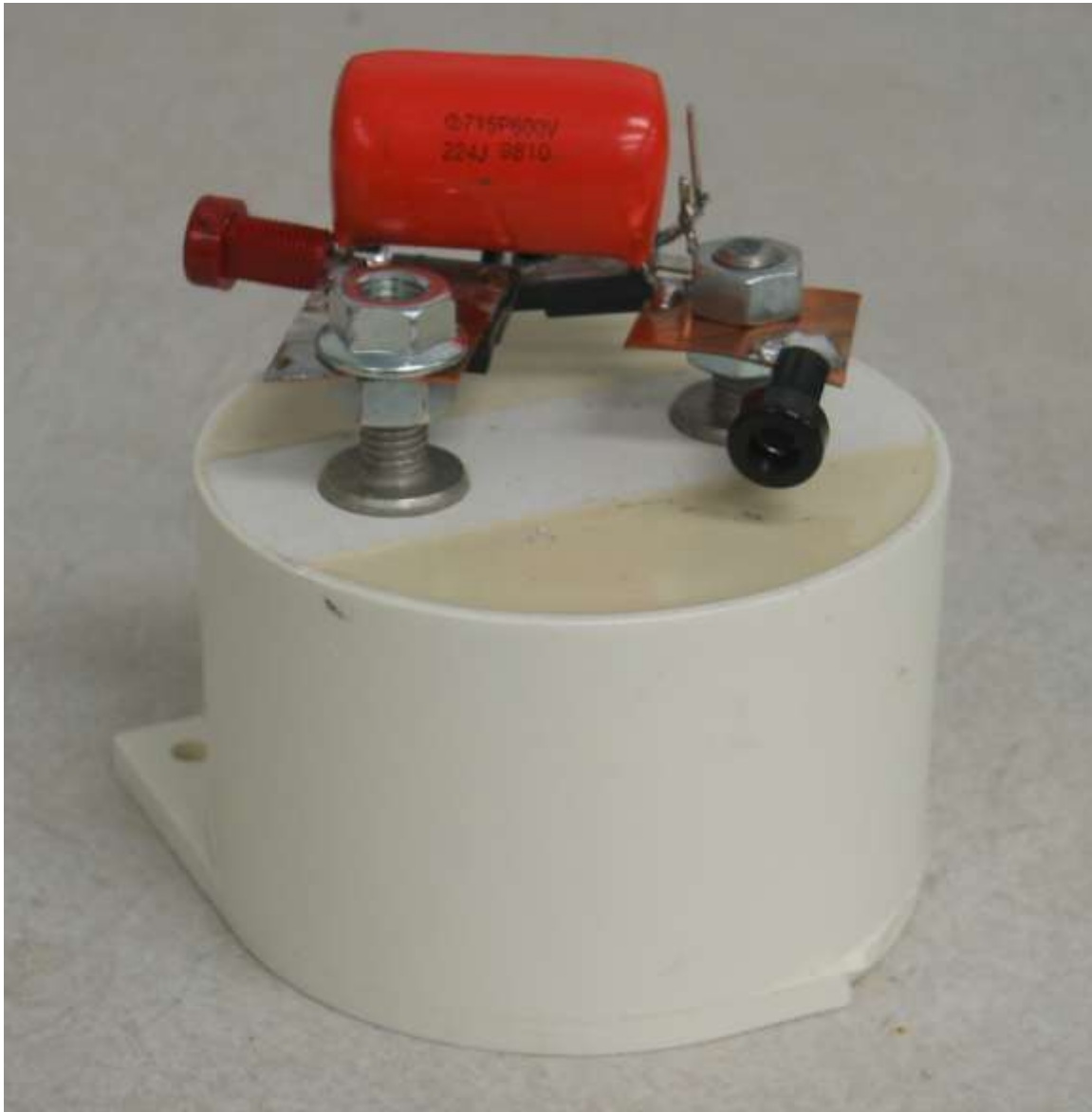
Figure 30: Vishay GLI capacitor with CoolMOS and ultra-fast EPU06 diode and Vishay Orange Drop bypass capacitor
