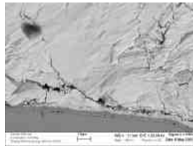
Figure 3.2-1: Severe cracking was not observed in the Sn/37Pb samples.
