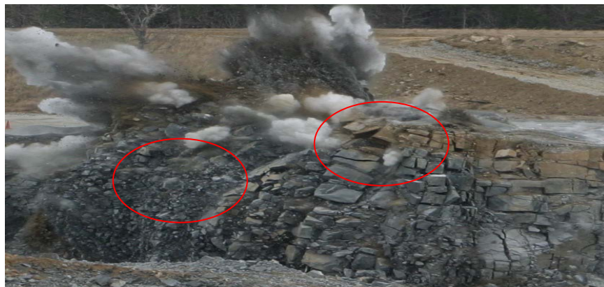
Figure 4.5 Liberated versus broken rock in the Pittsboro blast (JKMRC, 1996)
