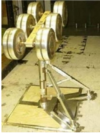
Figure 1.1: Low Fidelity 26% Scale Model of the 777 Main Landing Gear (Truck Angle = 0 deg.)
