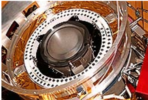
Figure 1.1: The NSTAR thruster mounted on the Deep Space 1 spacecraft.
