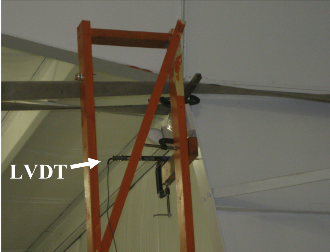
Figure 7-8: Location of Linear voltage displacement transducer
