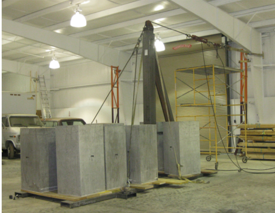
Figure 7-3: Load frame and rigging assembly
