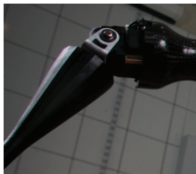
Figure 2.5: The distal joint also provides support on both sides of the actuator, similar to the revolute joints two and three of the proximal joint. Courtesy Virginia Tech. Photograph taken by Josh Armstrong.
