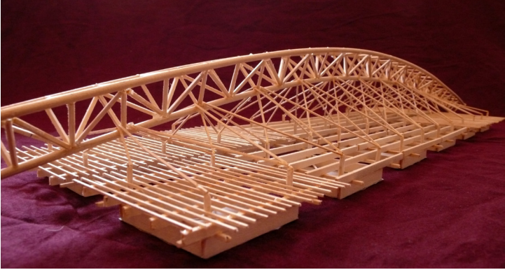
roof truss model from above model showing the cable lattice work that connects the arc and suspended louvers.
