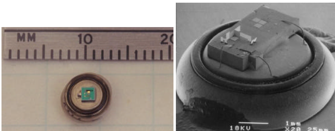
Figure 1.2: 63 \text{ mm}^3 mote with a MUMPS optics chip containing a CCR for communication, a CMOS ASIC for control, and a hearing aid battery for power. [from http://www-bsac.eecs.berkeley.edu/~warneke/SmartDust/index.html ]
