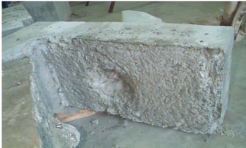
Figure 4.6 Concrete pry-out failure.
