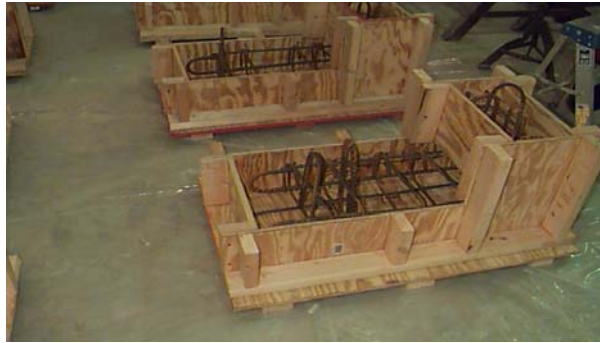
Figure 3.10 Extended double leg stirrups used as shear connectors.
