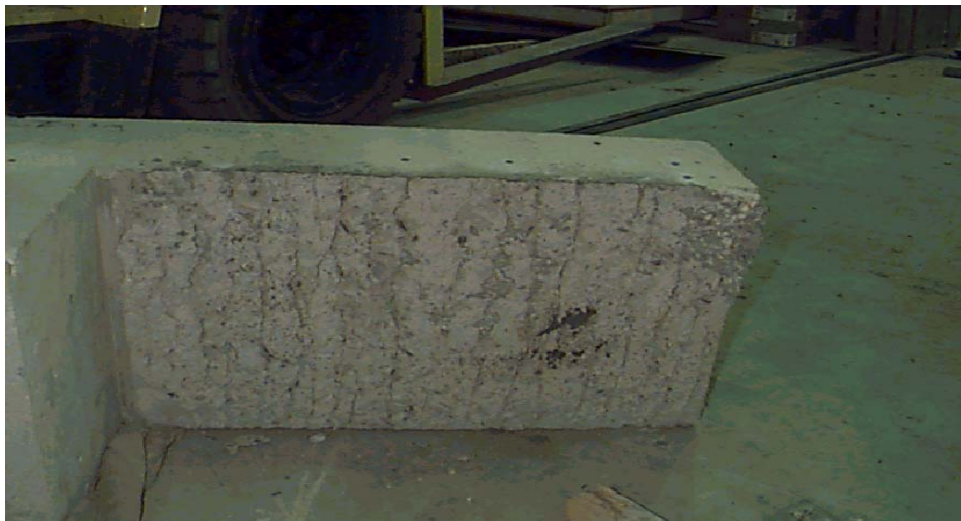
Figure 3.4 The raked surface of the beam element.
