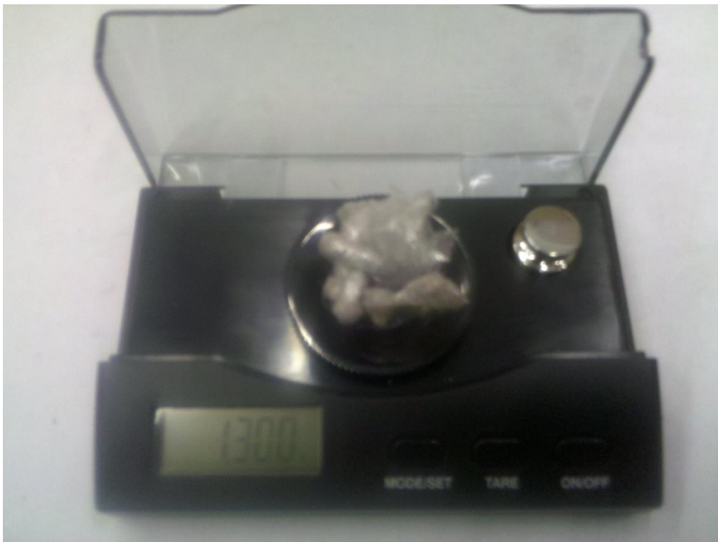
Figure 3.4. Photograph of scale used to measure mass of deposited particles
