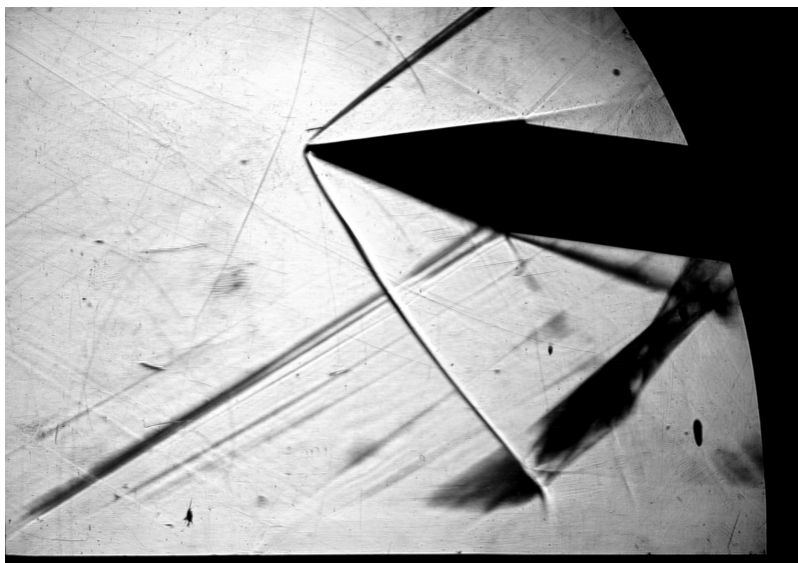
Figure 50: Schlieren photographs of the SSWT wedge constellations
