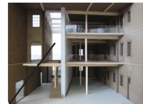
Sections of the second and third floors were cut back to create a multi-story atrium allowing transparent circulations from the basement to the third level and creating a visual vertical continuity that the previous space lacked.
