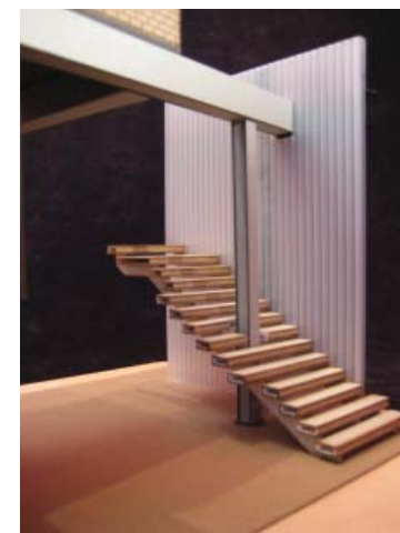
The placement of this existing column was incorporated into the new main level stairway as a nod to its structural importance and in an effort to force the visitor to engage the old building in an unexpected manner.
