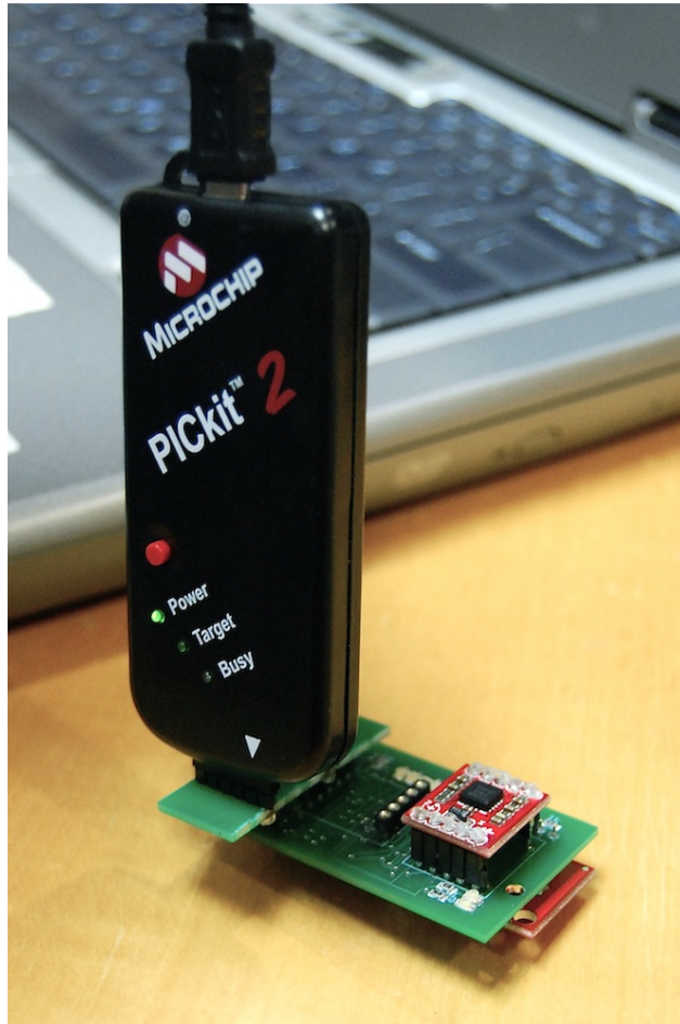
Figure 4.1: A Tier 1 sensor’s PIC being programmed by the PICkit.
