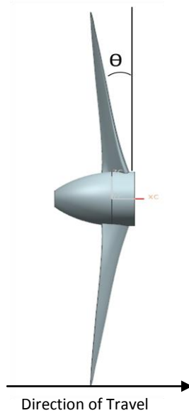
Figure 3-2: Propeller rake, \theta
