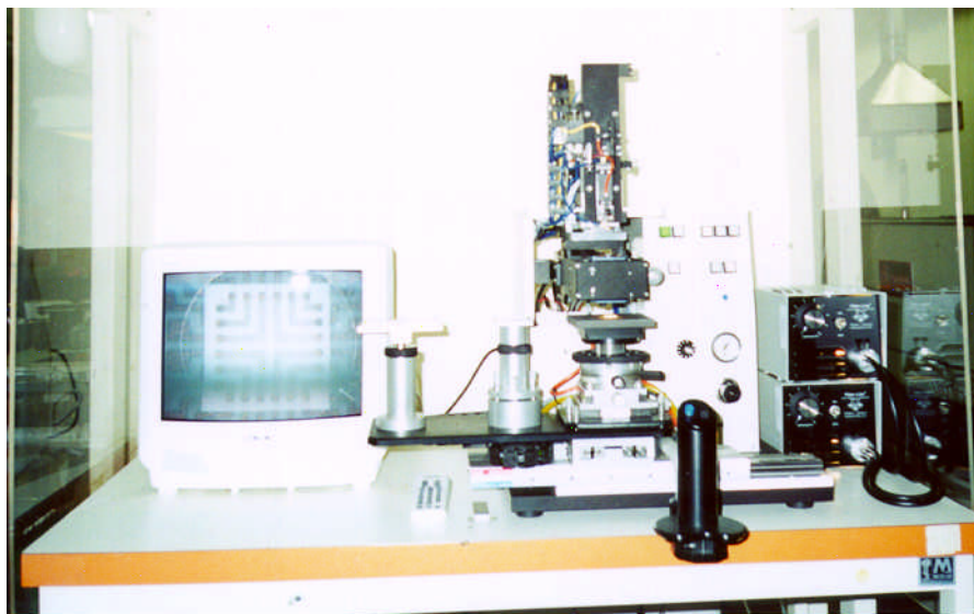
Figure 3.3 a) The table top Flip Chip placement system-Model 850 (from Semiconductor Equipment Corporation).
