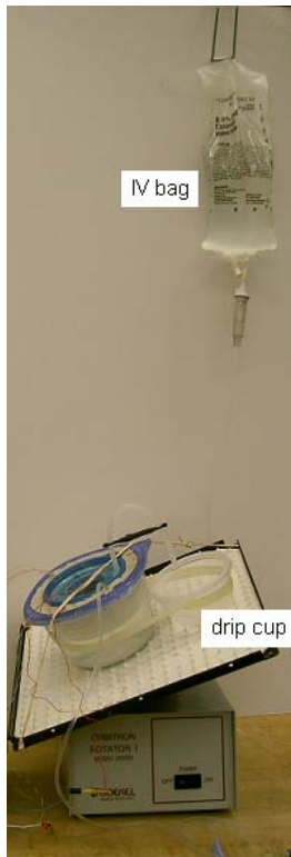
Figure 6.10. Orbitron IV drip test stand. The drip cup collected water leaving the phantom and was measured at the end of the test to find the average flow through the test stand. The hanging IV bag creates the potential for water to flow through the stand.
