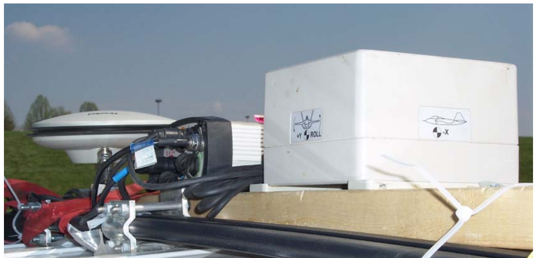
Figure 3.3: Rover Instrumentation (a) A Ford Excursion acted as the rover. (b) Three of the GPS receivers were located in the back seat. (c) The GPS antenna, fourth GPS receiver, and IMU were located on the roof.
