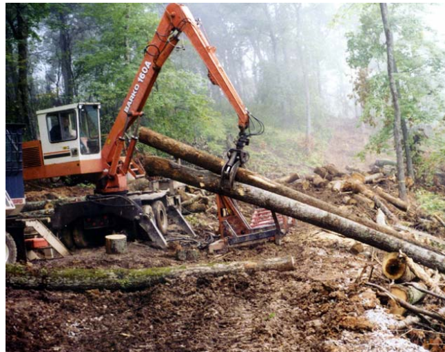
Figure 6: Poor location of the loader resulting in operational delays when loading the truck
