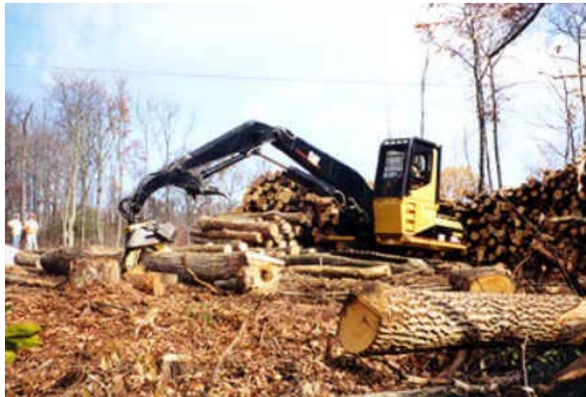
Figure 9: CAT 320B shovel excavator with a Hultdins 32-inch grapple saw at the main cable landing
