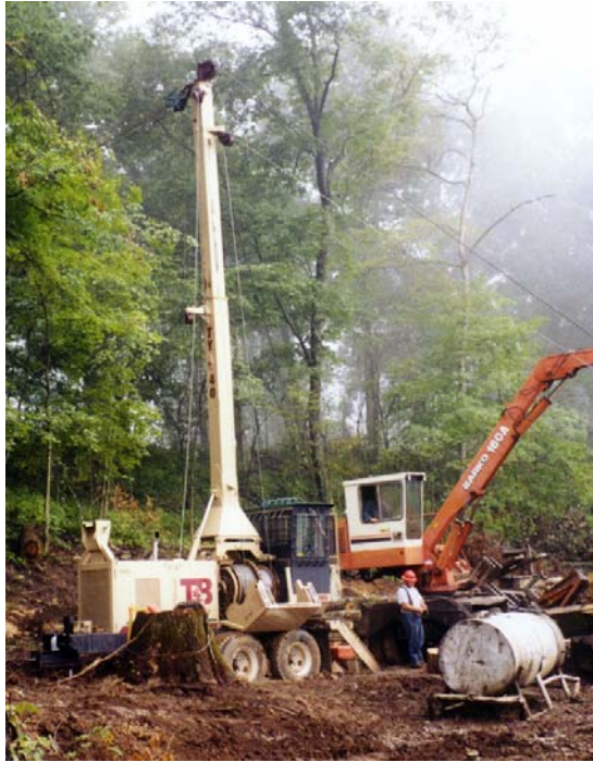
Figure 2: Wes Hood Logging: Thunderbird™ TY40 yarder with Barko 160A loader.
