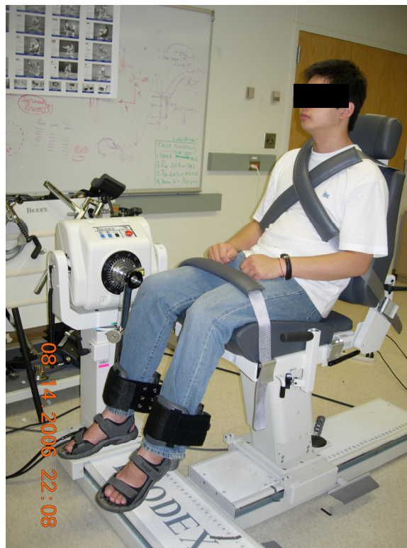
Figure 2.3. Biodesx Set up for the isokinetic bilateral fatigue exertions
