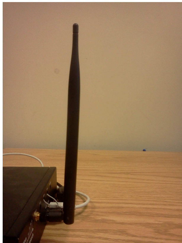
Figure 4.2: Antenna used on the transmitter and receiver (VERT900)
