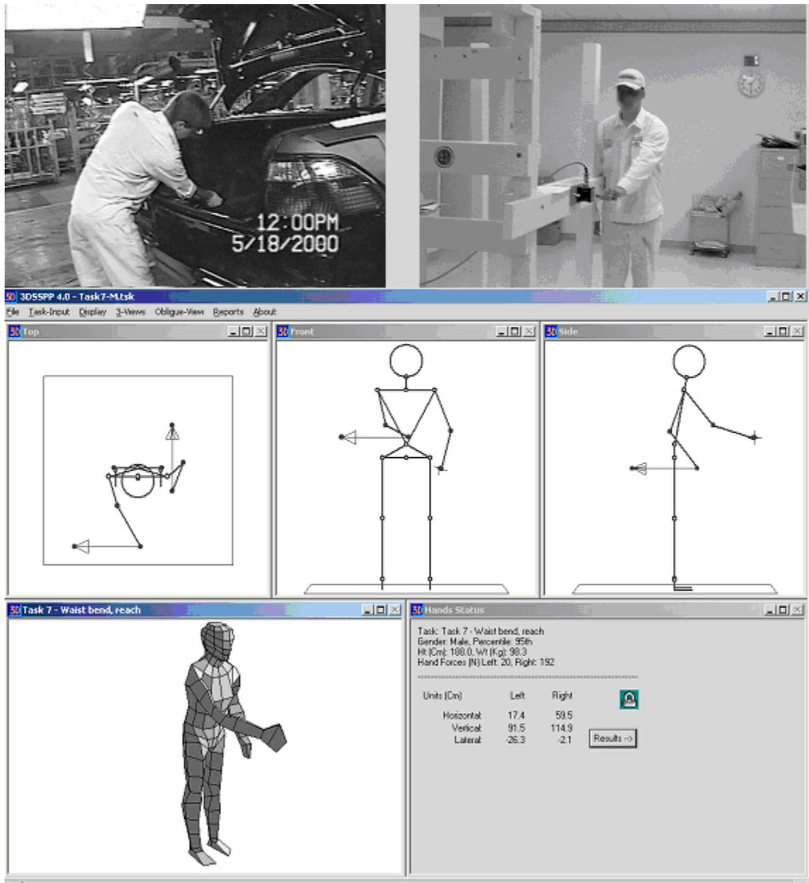
Figure 14. Observed task (top left), experimental simulations (top right), and 3DSSPP model (bottom) for tasks 7 and 8
