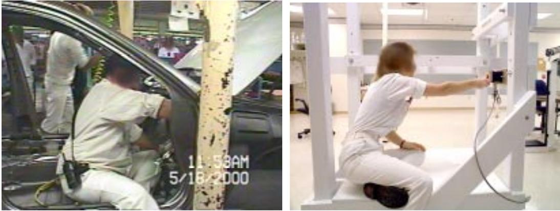
Figure 23. R/S Grommets operation (left) and experimental configuration (right). This was simulated as Task #9 and #10: Seated Forward Reach, Index and Thumb Couplings (Thumb shown).
