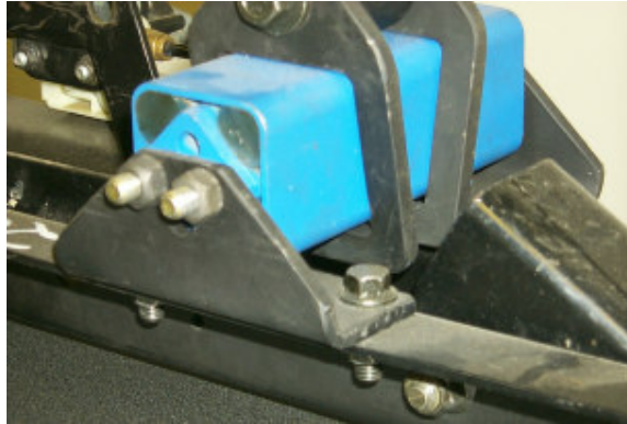
Figure 2-9. Elastomeric Torsion Spring of Prototype Suspension
