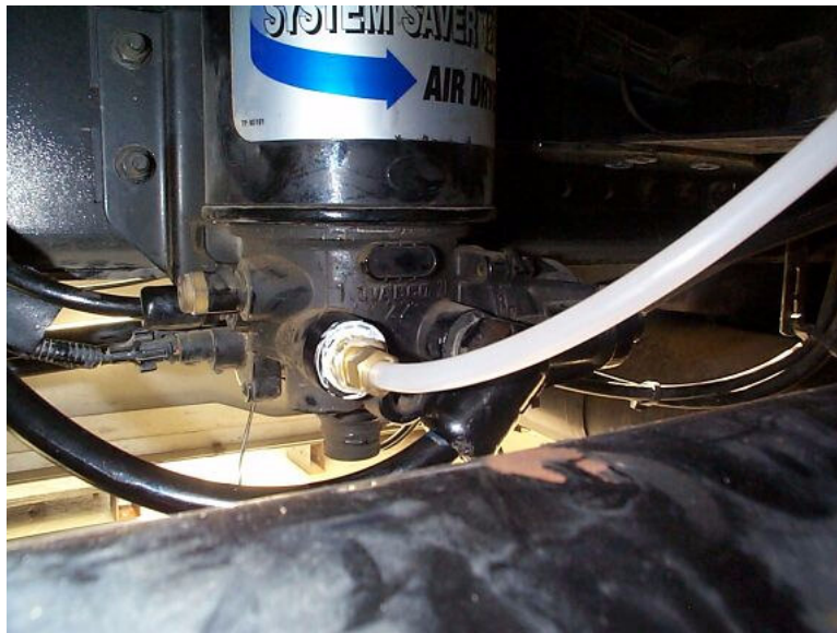
Figure 3-7. Air Dryer with Inlet Bypass Hose
