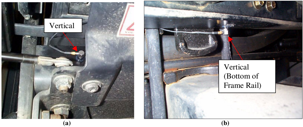
Figure 3-17. Frame Accelerometers (a) at Front and (b) at Second Axle
