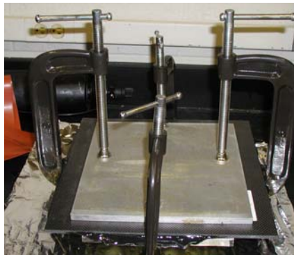
Figure 3.3. Clamping with aluminum plates
