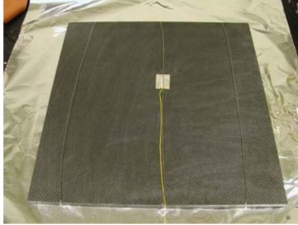
Figure 3.2. Bondline thickness wires and thermocouple placement
