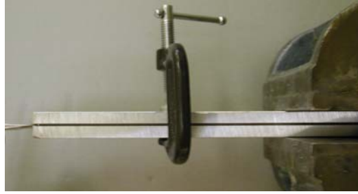
Figure 3.4. Aluminum specimen precracking using a C-clamp to force arrests
