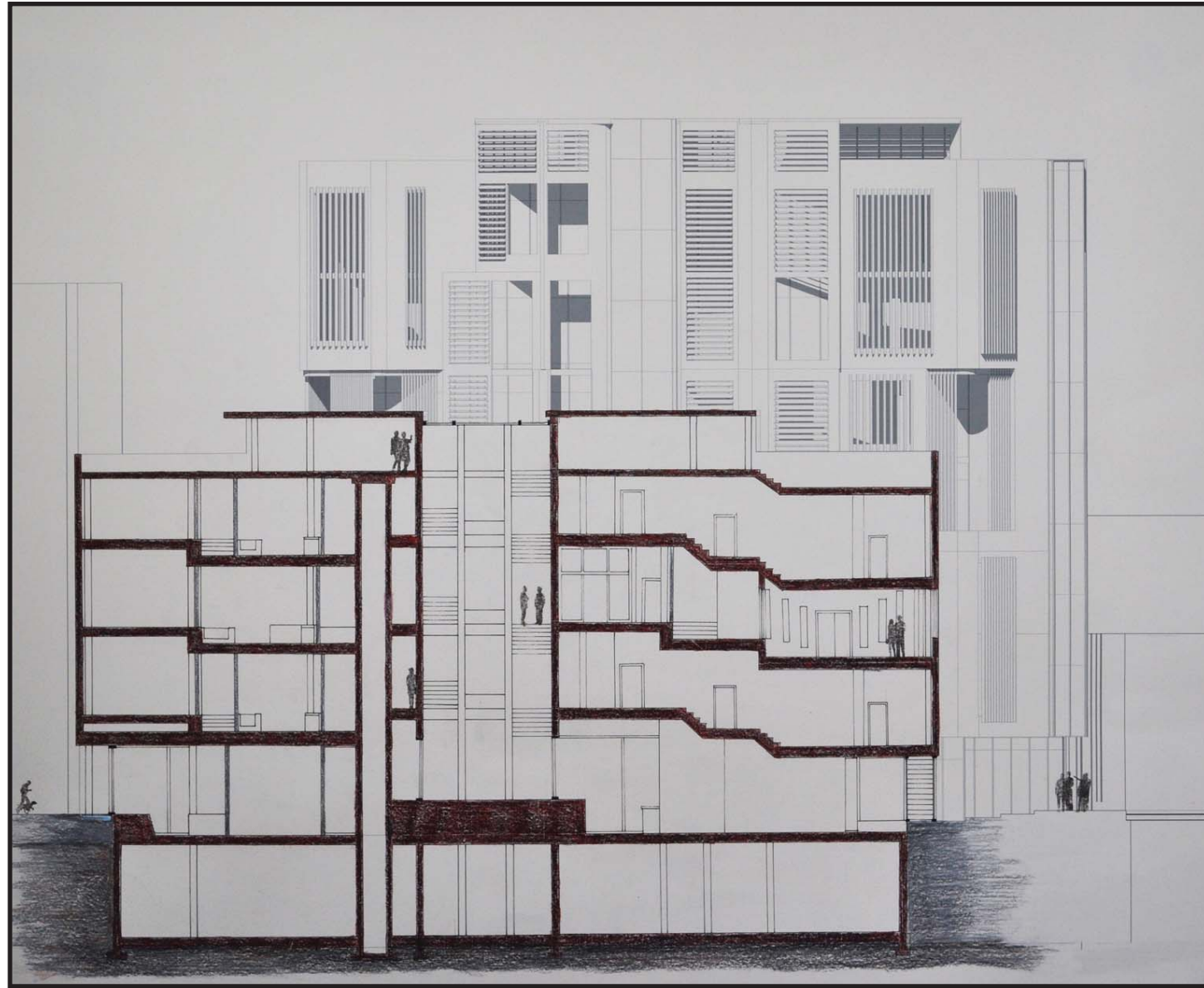
hotel section: expressing elevation changes within the common areas while maintaining subtle and singular changes within each dwelling unit
