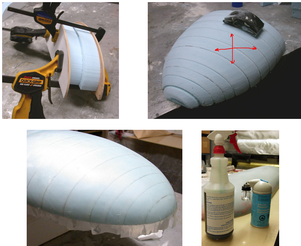
Figure 2.5: (Top Left) Gluing the Cross-Sections Together, (Top Right) Sanding the Plug to Its Proper Shape, (Bottom Left) Adhering the Fiberglass Weave to the Foam, (Bottom Right) The Finished Plug after Applying the Polyvinyl Alcohol Layer
