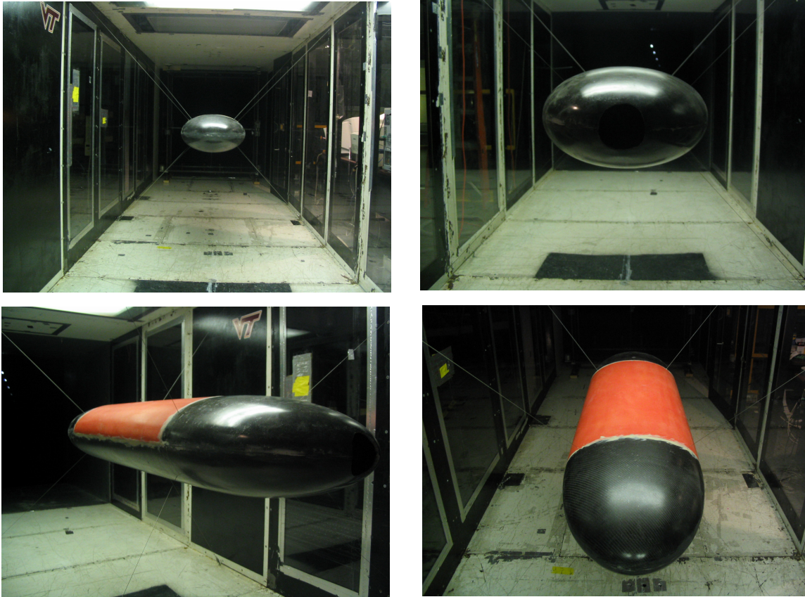
Figure 3.3: Model Mounted in Tunnel with the X Guy Wire Configuration
