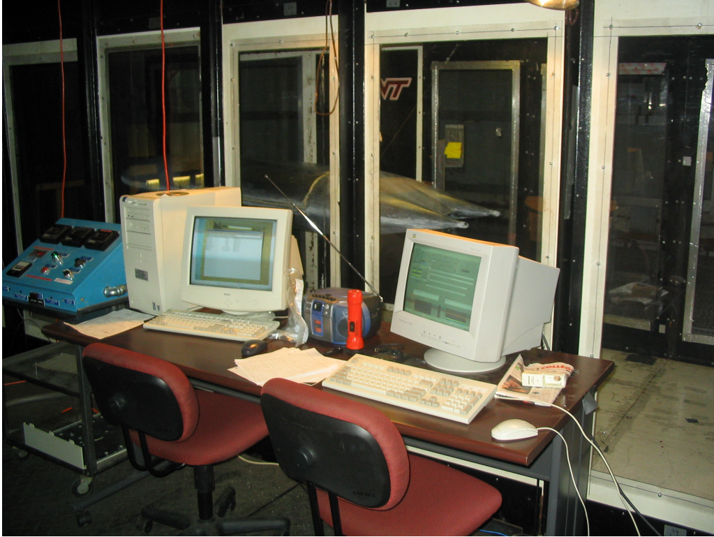
Figure 2.11: Data Acquisition and Tunnel Control Station, with NNEMO Model in Background
