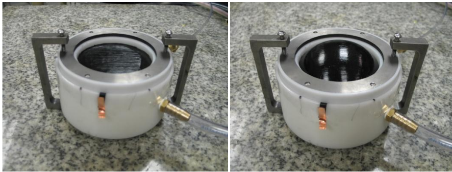
Figure 16. Actuator before and after inflation.
