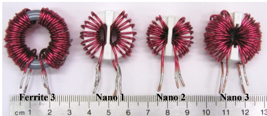
Fig. 5-3: CM choke representation using ferrite and nano-crystalline core
