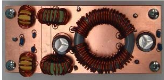
Fig. 4-20: EMI filter layout with two point ground
