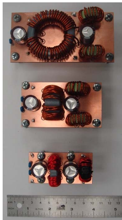
Fig. 5-14: Filter reduction when CM choke is improved
