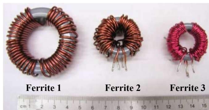
Fig. 5-13: CM chokes comparison after multi-layers winding and higher current density
