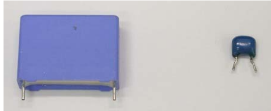
Fig. 3-16: Size representation of film (left) and ceramic (right) capacitors for CM filter
