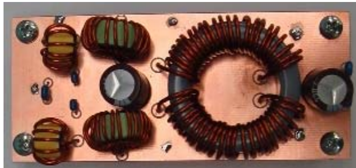
Fig. 4-18: EMI filter layout with one point ground
