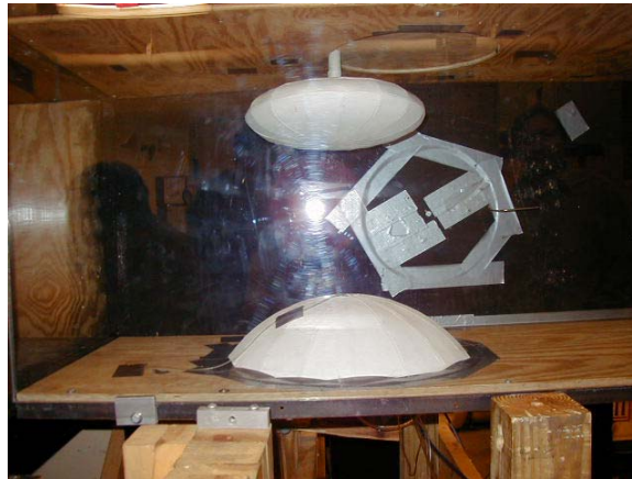
Figure 3.9 - Experimental setup with ellipsoid suspended from top of wind tunnel - Scenario 2
