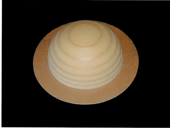
Figure 3.12 - MDF base with chipboard flange, used as a mold for high-impact polystyrene lower hemisphere
