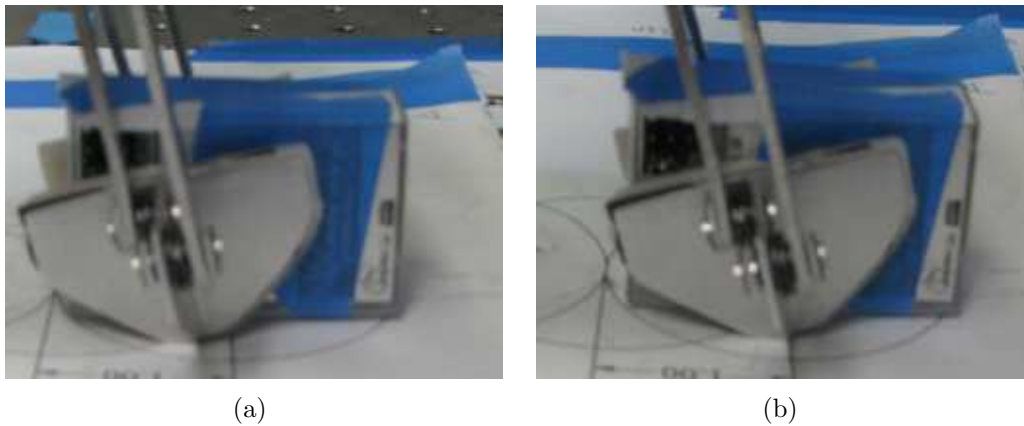
Figure 5.16: End effector grabbing a block 50 mm away from front lip of the sampling tray. Figure (a) shows a grab without correction while (b) shows a grab with a correction factor added. The corrected grip position is closer to the center of the object
