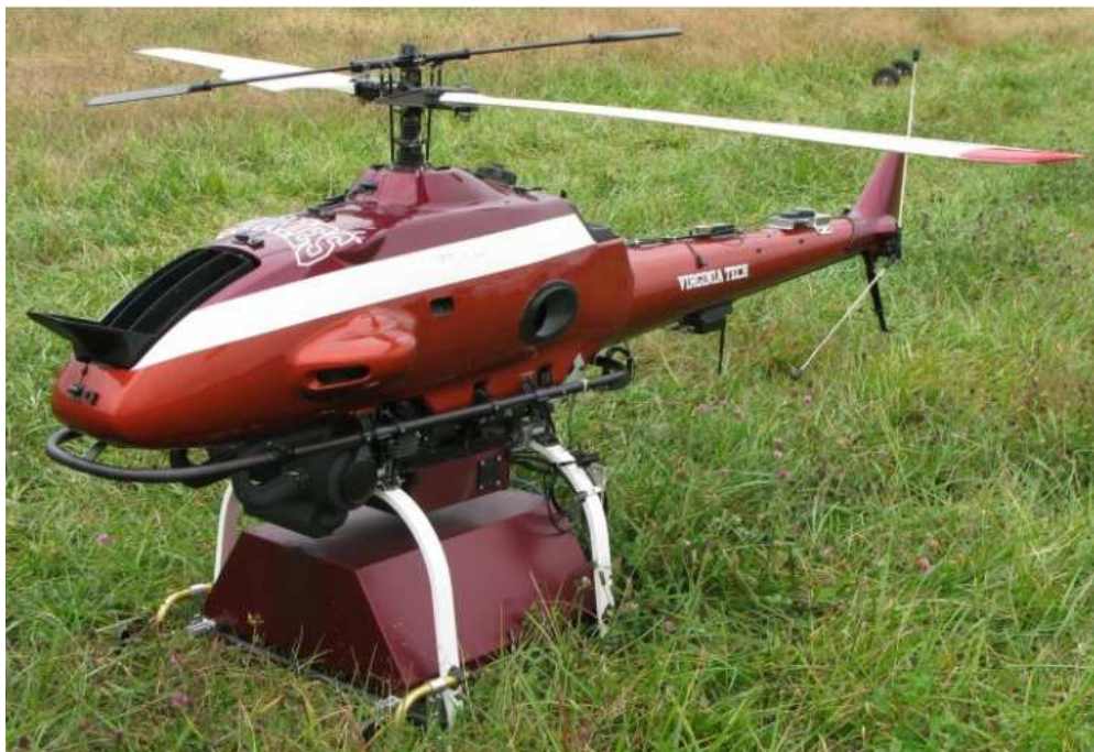
Figure 1.2: The Yamaha RMAX retrofitted as a UAV at the Unmanned Systems Lab.
