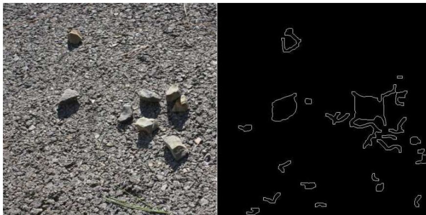
Figure 4.3: Rockfinder demonstration on an image. On the left there are 8 rocks strewn on pavement and on the right is the binary image that is the result of the Rockfinder code.
