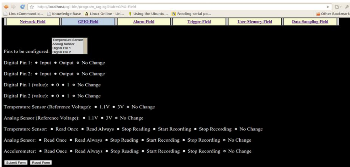
Figure 5.4: GUI to program the GPIO field parameters of the tag
