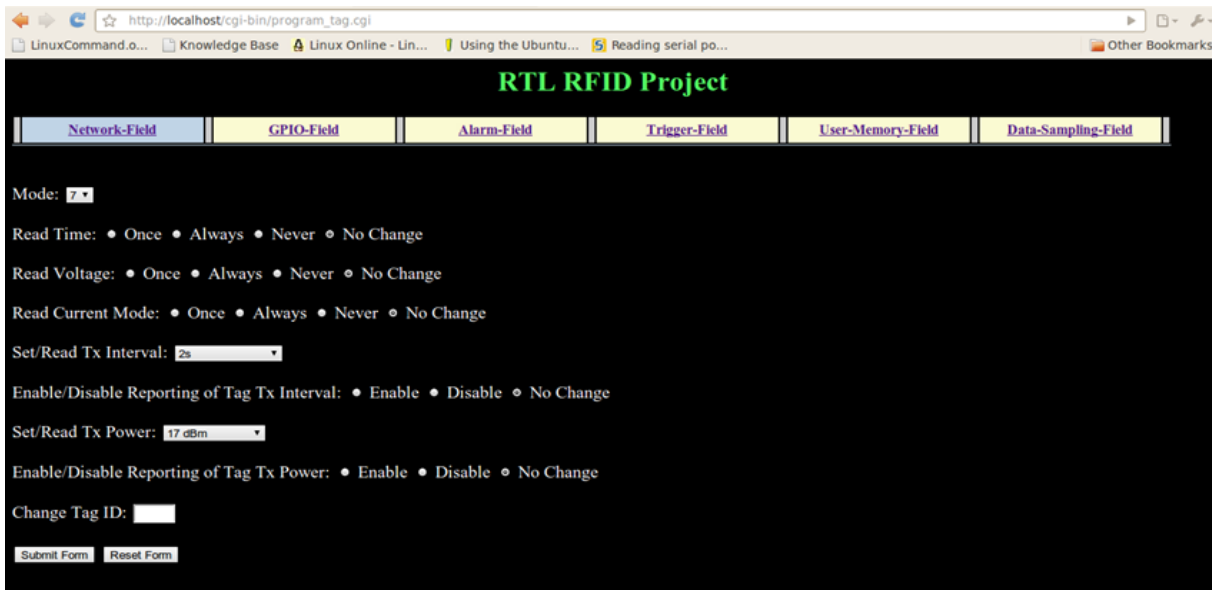
Figure 6.17: GUI used to set the transmission related parameters for a particular mode
