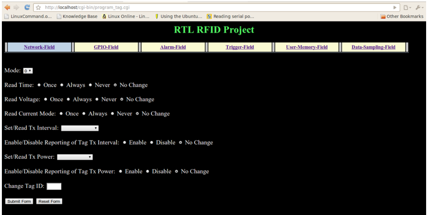
Figure 5.3: GUI to program the network field parameters of the tag
