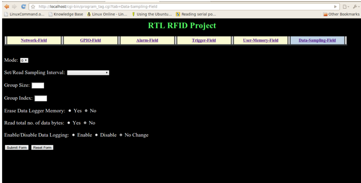
Figure 5.8: GUI to program data sampling field parameters of the tag
