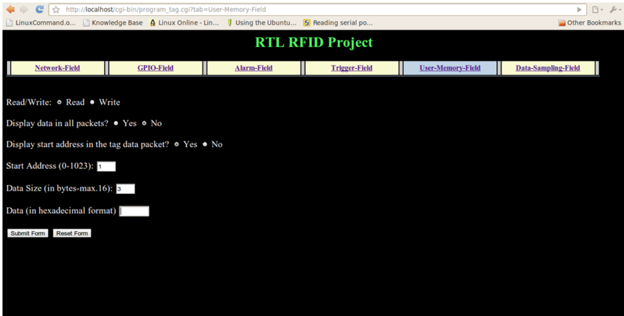
Figure 6.22: GUI to read data from the EEPROM memory inside the tag
