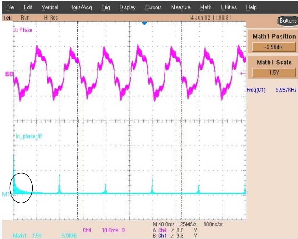
Figure 29 Current FFT for 120.3 in-lb, 1000 RPM, and 10 kHz Switching
