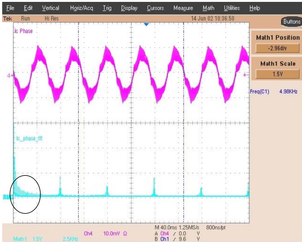
Figure 48 Current FFT for 120.3 in-lb, 2000 RPM, and 5 kHz Switching
