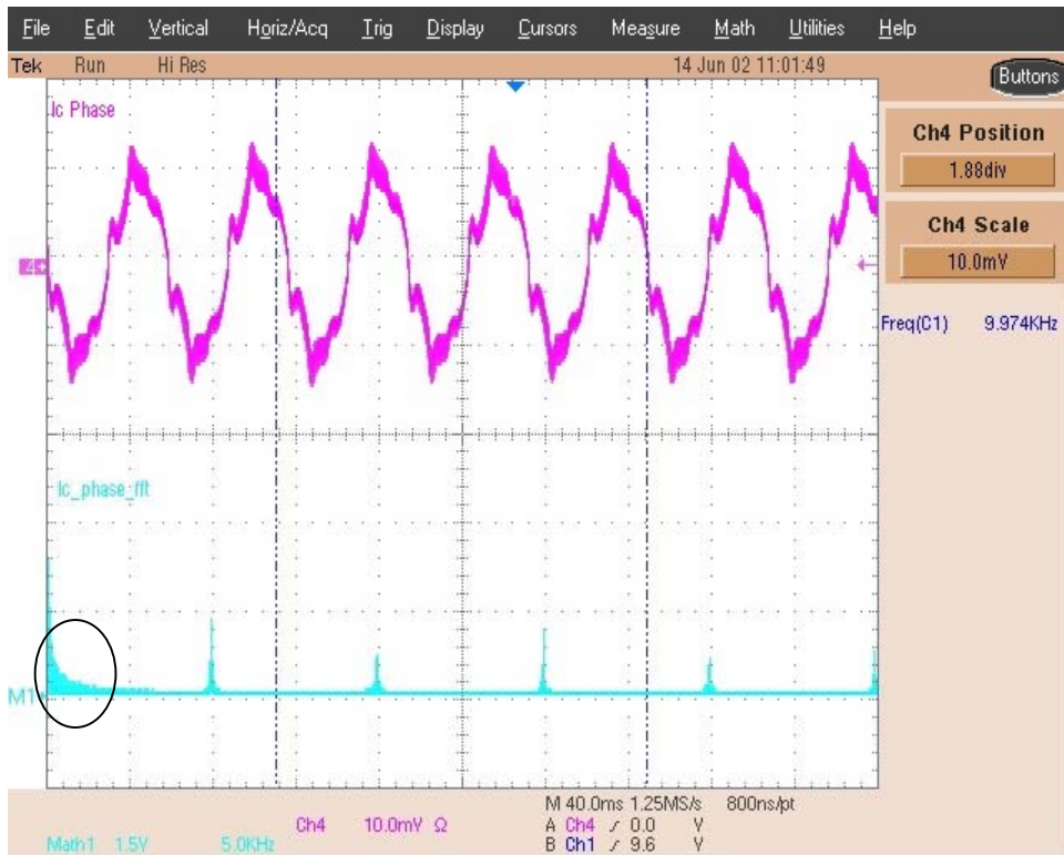
Figure 51 Current FFT for 180.0 in-lb, 2000 RPM, and 10 kHz Switching
