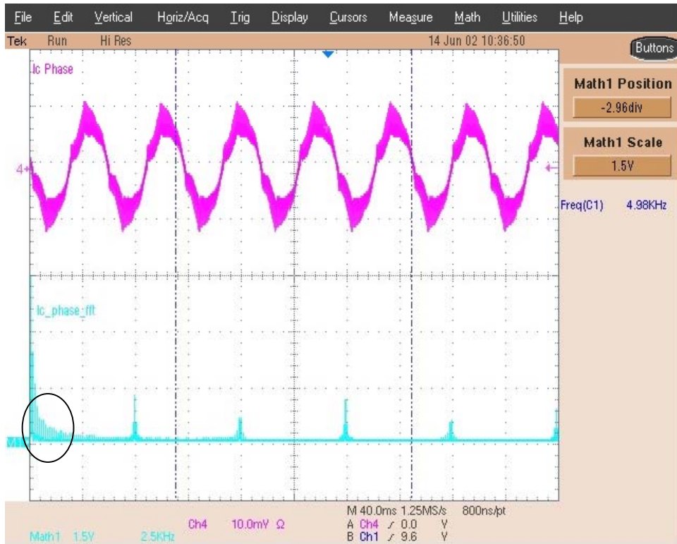
Figure 30 Current FFT for 120.3 in-lb, 1000 RPM, and 5 kHz Switching
