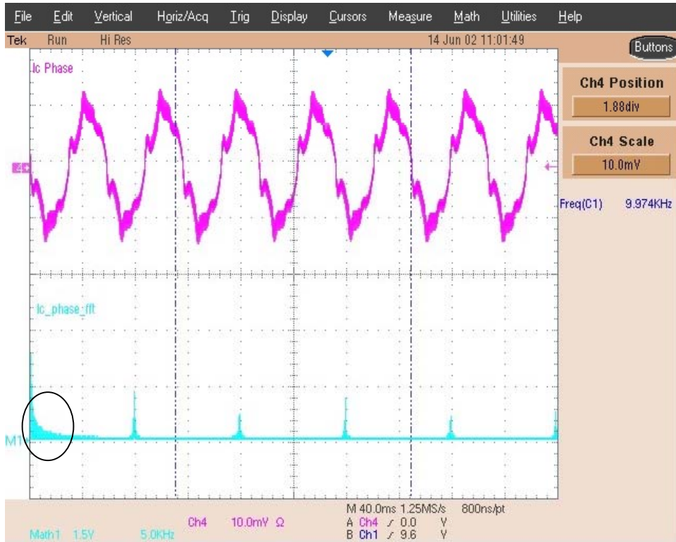
Figure 69 Current FFT for 180.0 in-lb, 3000 RPM, and 10 kHz Switching
