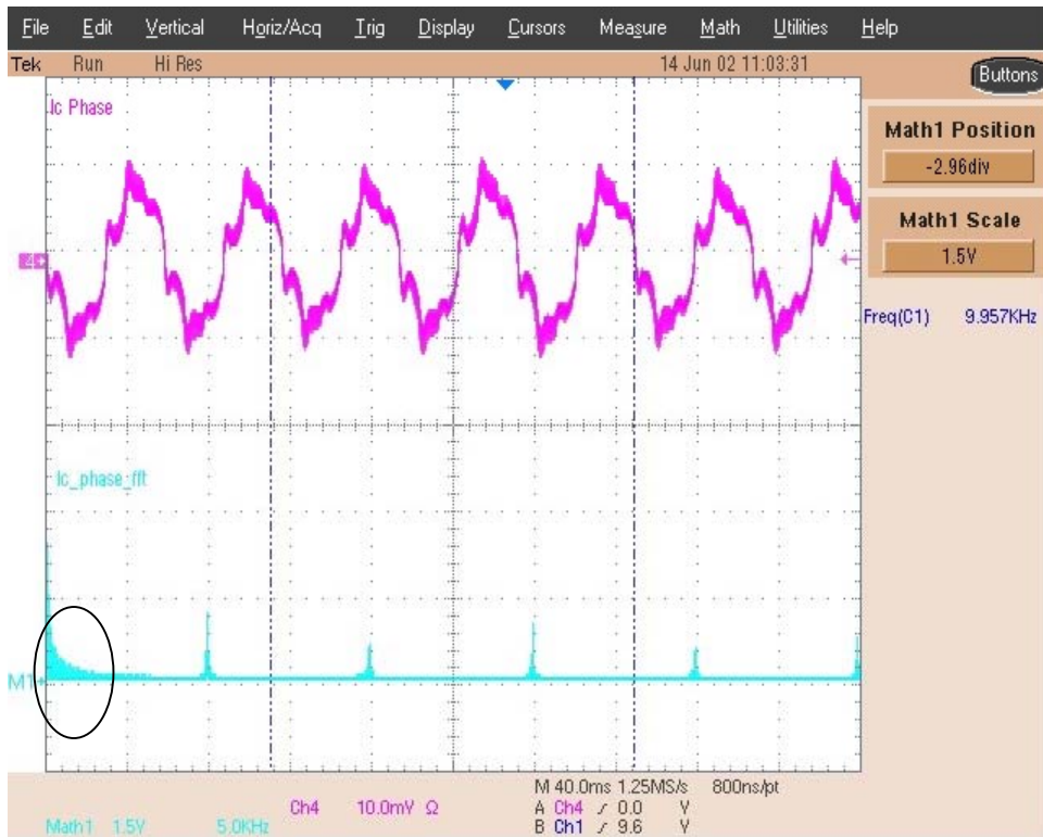
Figure 65 Current FFT for 120.3 in-lb, 3000 RPM, and 10 kHz Switching
