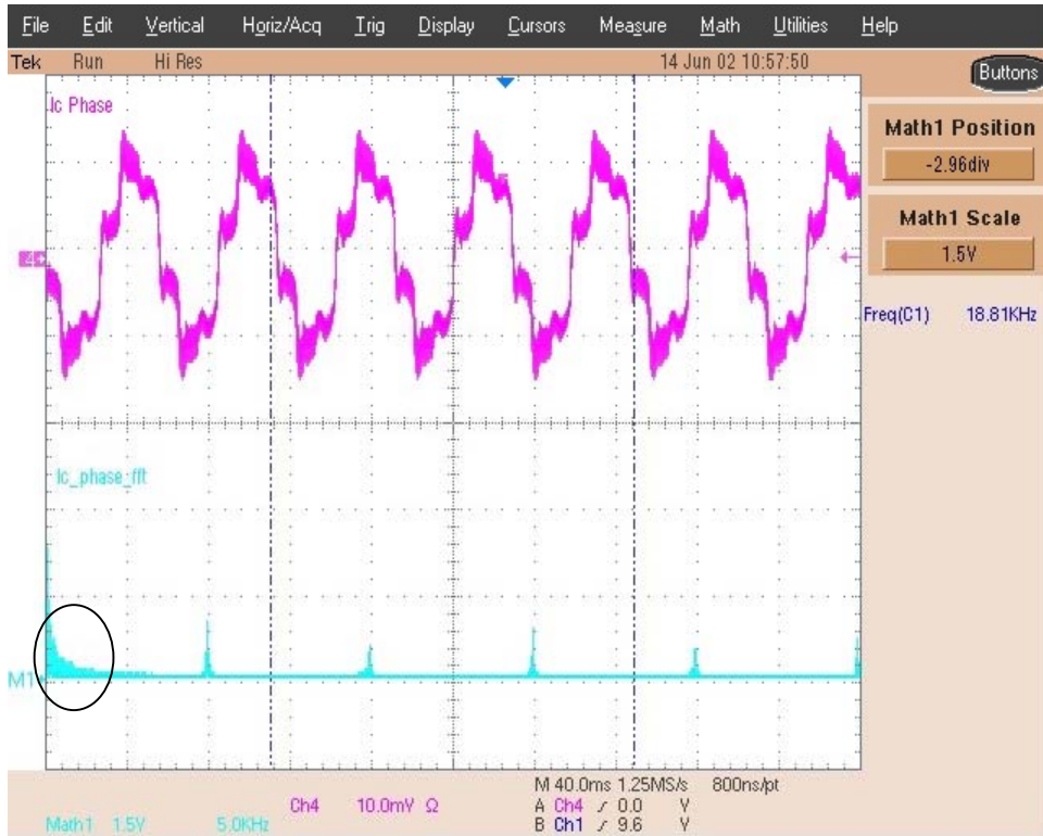
Figure 61 Current FFT for 60.5 in-lb, 3000 RPM, and 10 kHz Switching
