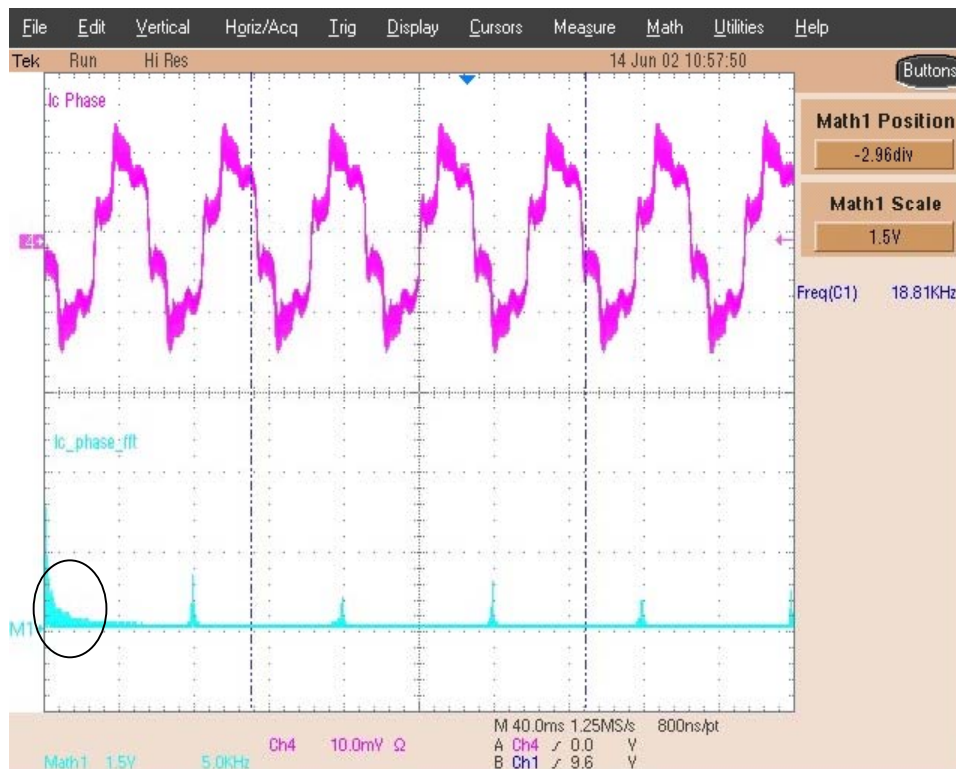
Figure 25 Current FFT for 60.5 in-lb, 1000 RPM, and 10 kHz Switching
