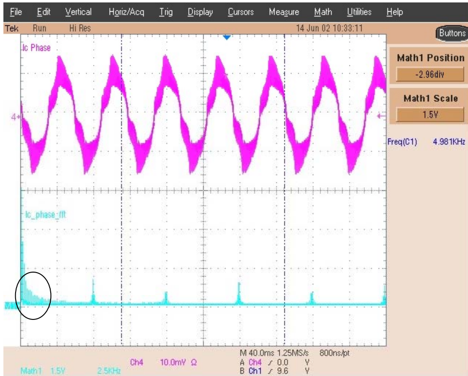
Figure 62 Current FFT for 60.5 in-lb, 3000 RPM, and 5 kHz Switching
