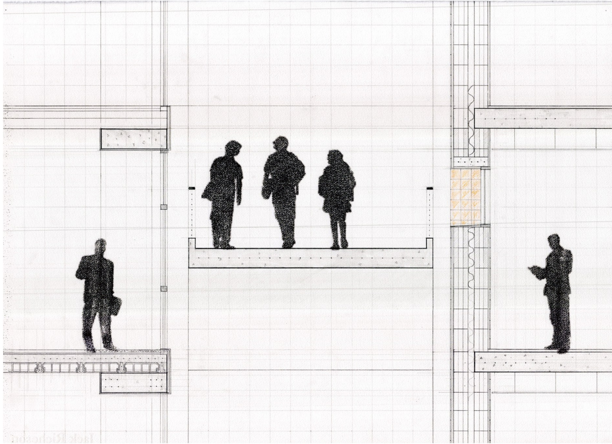
Figure 74: Section detail at ramp and adjoining facades
