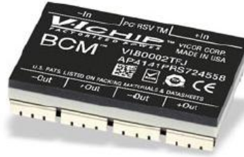
Figure 5.21: ZVS/ZCS sine amplitude converter VIB0002TFJ (source: www.vicr.com , 2010)
