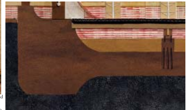
Fig. 64 Concrete base thick at rim; interior column is woven to base
