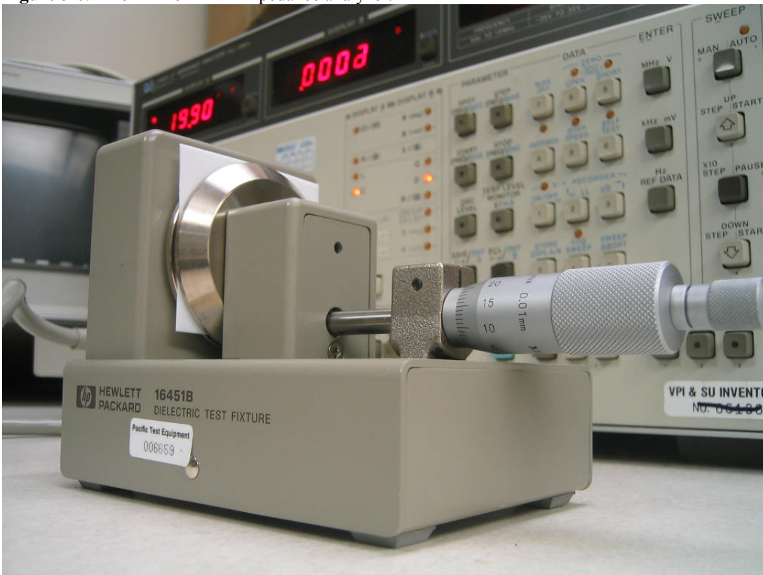
Figure 3-7. The HP16451B dielectric test fixture. The guarded electrode configuration greatly reduces the fringing of the electric field at the edge of the parallel-plate structure.
