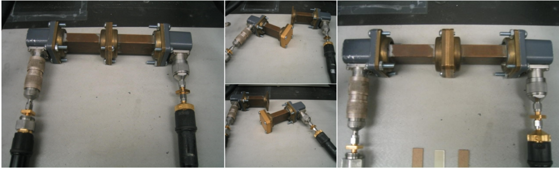
Figure 4-19. The TRL calibration process. After connecting the thru, reflect, line, and isolation standards, the network analyzer computes the 12 error coefficients for direct viewing of S-parameters.
