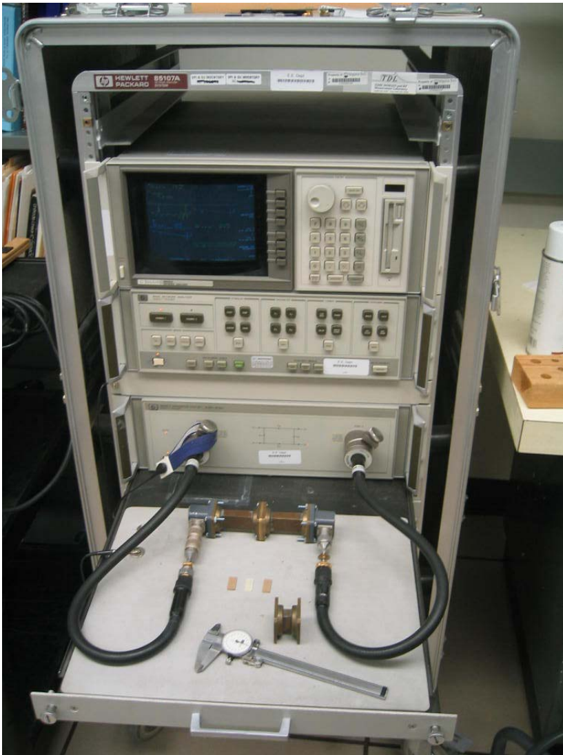
Figure 4-18. The HP 8510C Vector Network Analyzer (VNA). The measured S-parameters are transferred to a computer, where the matlab code is run to solve for the complex permittivity.
