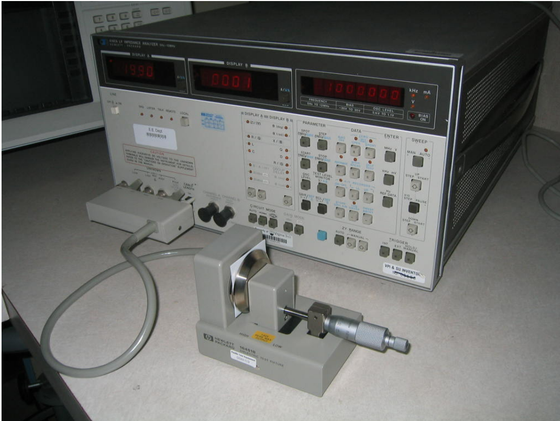
Figure 3-9. The capacitive measurement setup with Teflon sample. 1m cable compensation is provided by the 4192 to reduce the effects of the test fixture leads.
