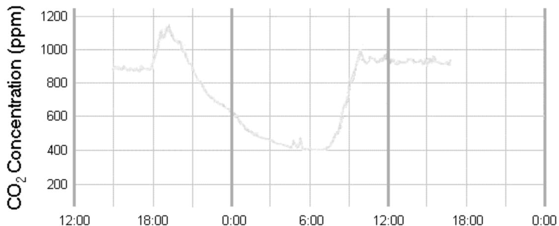
**Figure 4** Diurnal carbon dioxide fluctuation of an occupied office building.
