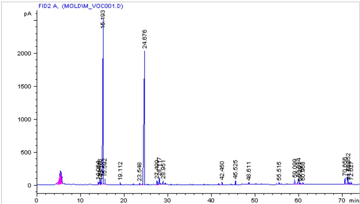
**Figure 14** Chromatogram for the back sample tube collected from purge air flowing over common grain mold growing on whole wheat bread. This illustrates breakthrough of the lighter compounds.
