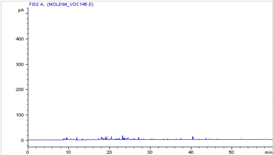
**Figure 23** Chromatogram for sample tube I taken directly from the conditioning oven. Conditioned on 7/1/99 with graphite ferrules and an organic scrubber on the incoming nitrogen purge line.
