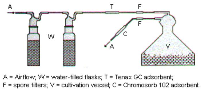
**Figure 2** Equipment for sampling volatiles from fungi cultivated on wheat. (Borjesson et al., 1989)
