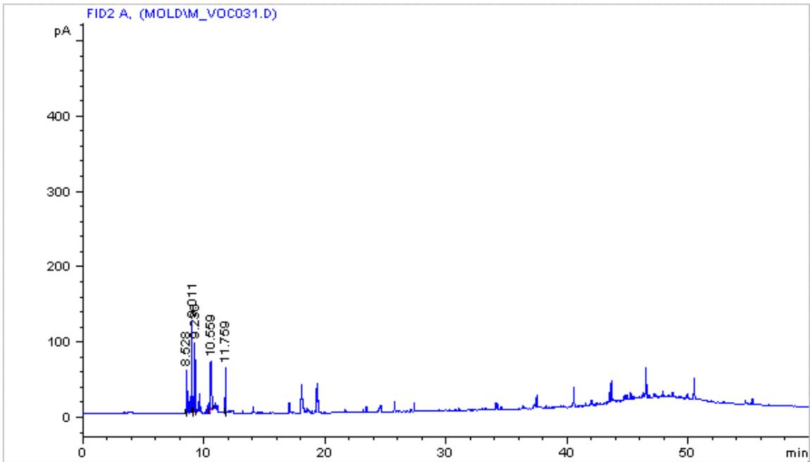
**Figure 21** Chromatogram for sample tube D taken directly from the conditioning oven. Conditioned on 4/22/99 with Teflon ferrules in the oven.
