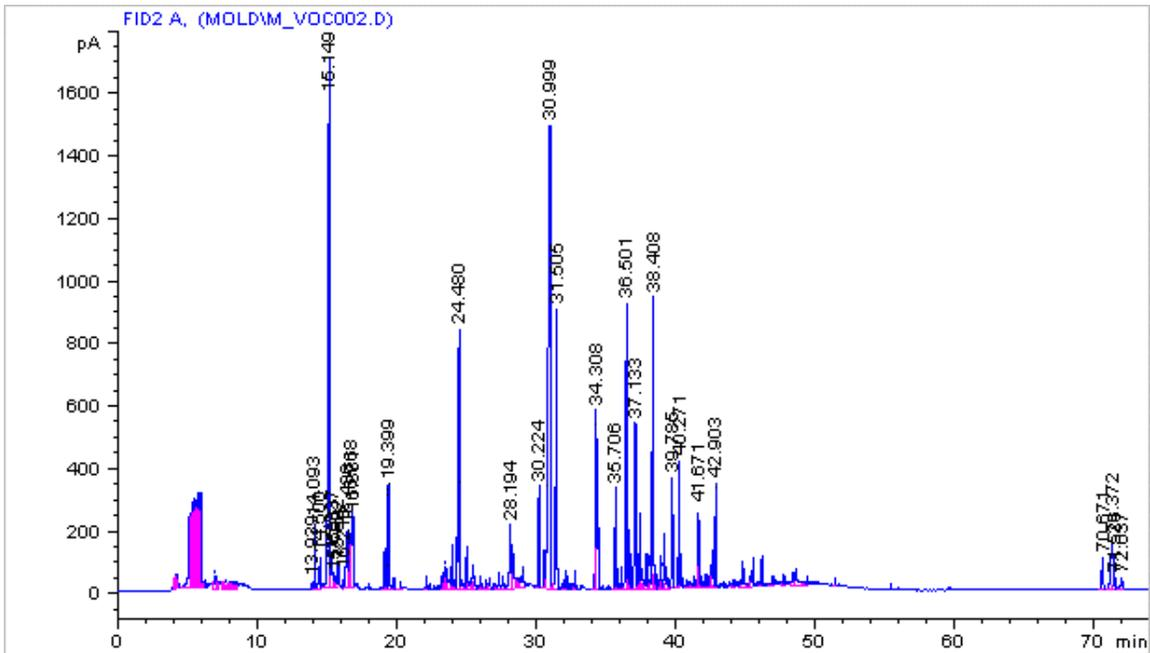
**Figure 13** Chromatogram for the front sample tube collected from purge air flowing over common grain mold growing on whole wheat bread. (23 hours, 14 ml/min)
