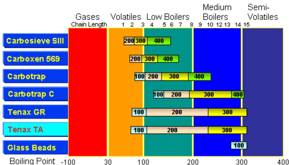
**Figure 11** Sampling ranges for adsorbent resins shown for alcohols methanol through pentadecanol. (Data provided by Scientific Instruments Services)
