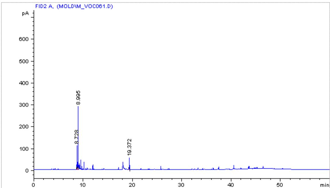
**Figure 18** Chromatogram for the back sample tube collected from purge air flowing at 15 ml/min over *Penicillium* growing on a dusty fiberglass filter for 24 hours on 4/27/99.
