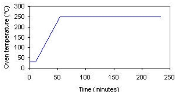
**Figure 9** Temperature profile of the method used to condition the desorption tubes.
