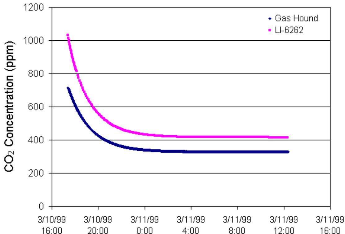
**Figure 28** Comparison of output from the LI-6262 and the LI-800, the Gashound.
