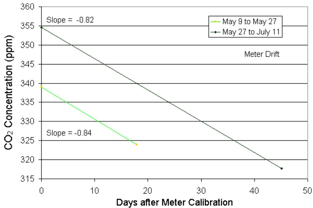
**Figure 30** Air tank readings before and after experimental runs showing the drift of the CO<sub>2</sub> meter.
