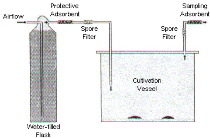
**Figure 3** Equipment for sampling volatiles from fungi cultivated on wheat. (Borjesson et al., 1990)
