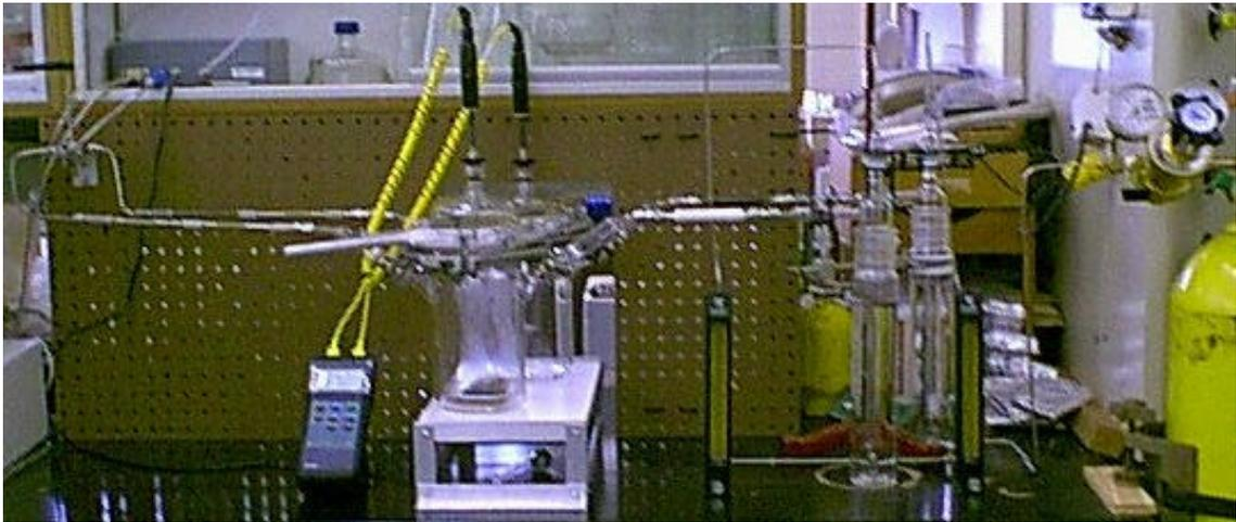
**Figure 10** Laboratory setup for the cultivation and monitoring of molds.
