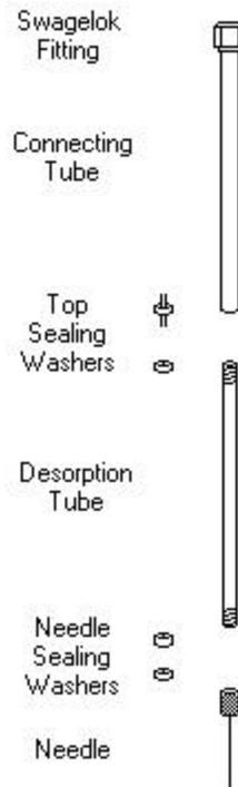
**Figure 35** Connecting diagram for the desorption tubes to the thermal desorption unit.
