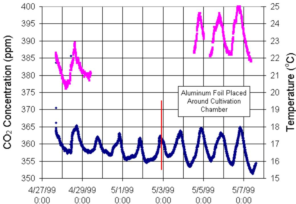
**Figure 32** Light / dark study of Penicillium on fiberglass filter#5 Temperature in pink and CO<sub>2</sub> concentration in dark blue. Airflow = 15 ml/min.
