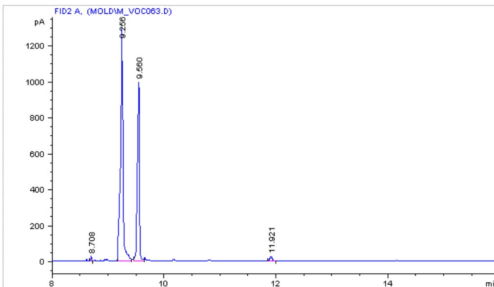
**Figure 34** Chromatogram for the standard composed of 0.02 ml and 0.01ml saturated headspace injections of 2-methyl-1-propanol and 2-pentanone respectively. (22°C and 720 mm Hg)
