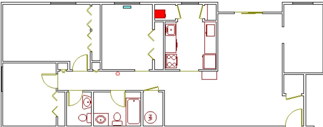
**Figure 39** The floor plan for 403 Hampton Court (1280 square feet 58x23) Ventilation system in red and sample collection and CO<sub>2</sub> monitoring point in blue.
