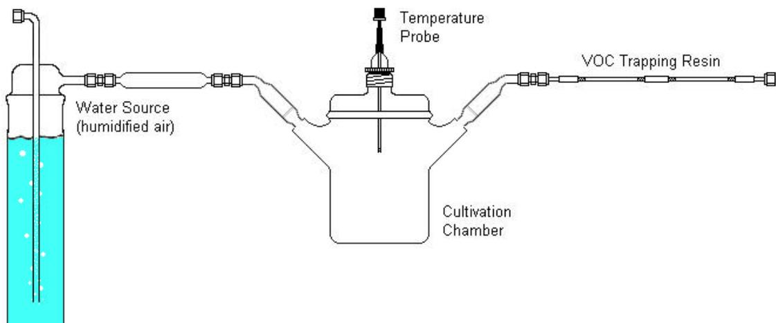
**Figure 6** Setup for the collection of volatile organics from cultured fungi.
