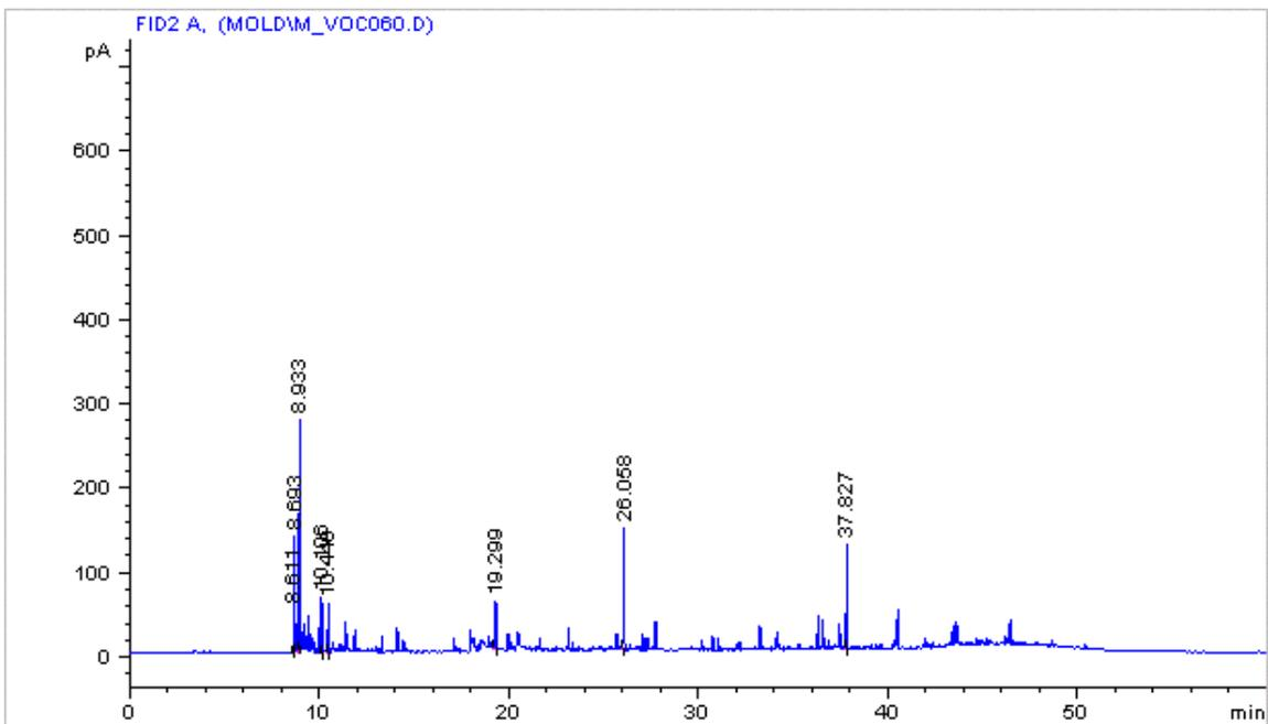
**Figure 16** Chromatogram for the front sample tube collected from purge air flowing at 15 ml/min over *Penicillium* growing on a dusty fiberglass filter for 24 hours on 4/27/99.
