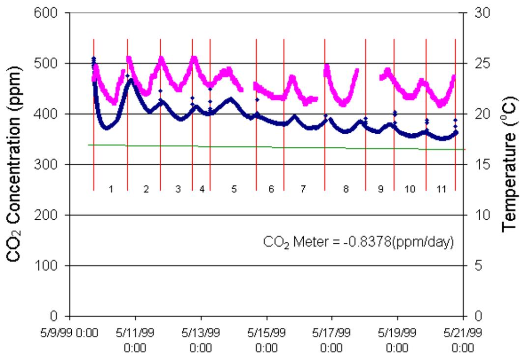
**Figure 33** *Penicillium* on fiberglass filter#1. Temperature in pink and CO<sub>2</sub> concentration in dark blue. Air tank CO<sub>2</sub> levels in green. Airflow = 14 ml/min.
