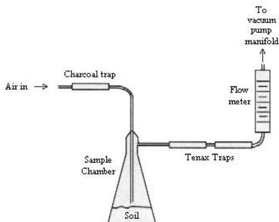
**Figure 1** Purge-and-trap apparatus for the collection of VOCs produced in soil microcosms. (Stahl et al., 1996)
