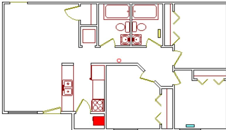
**Figure 40** The floor plan for 617 Lee St (824 square feet 38.5x22) Ventilation system in red, sample collection in yellow and CO<sub>2</sub> monitoring point in blue.
