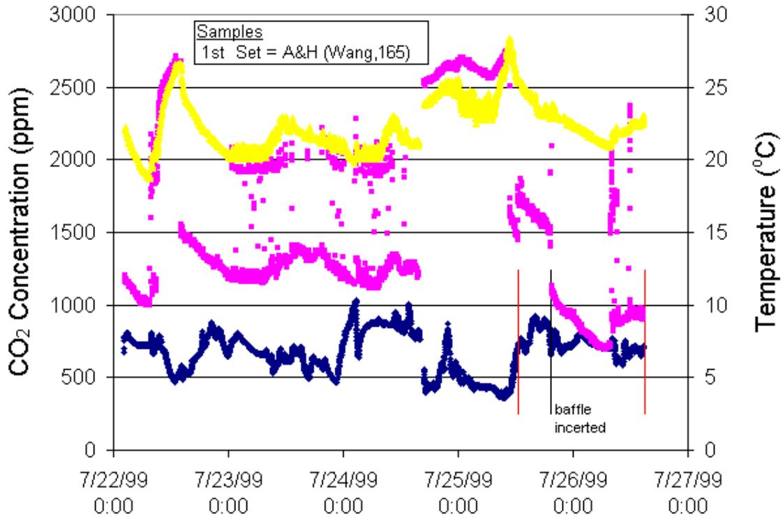
**Figure 41** Monitoring of temperature and CO<sub>2</sub> concentration at 403 Hampton Court. Yellow = Room Temperature; Pink = Duct Temperature; Blue = CO<sub>2</sub> Concentration
