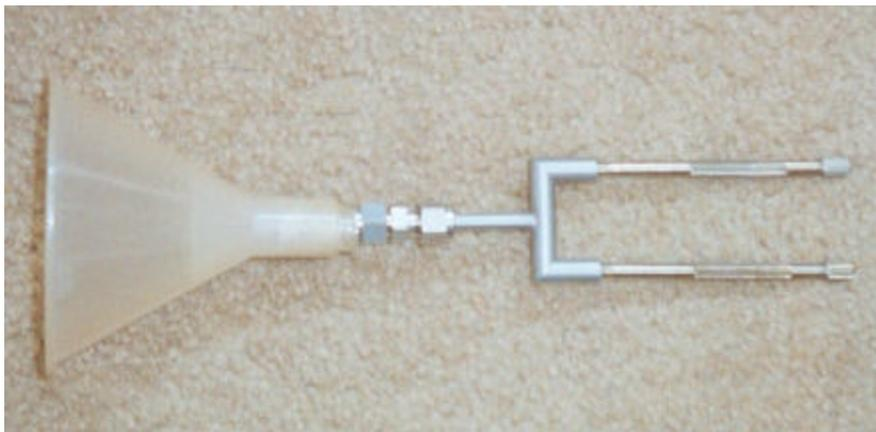
**Figure 43** Funnel technique used to collect ventilation samples.
