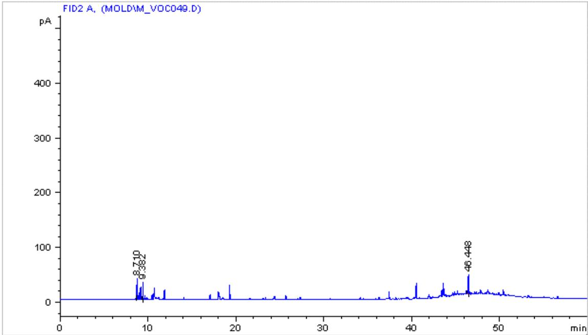
**Figure 22** Chromatogram for sample tube L taken directly from the conditioning oven. Conditioned on 4/29/99 with graphite ferrules in the oven.
