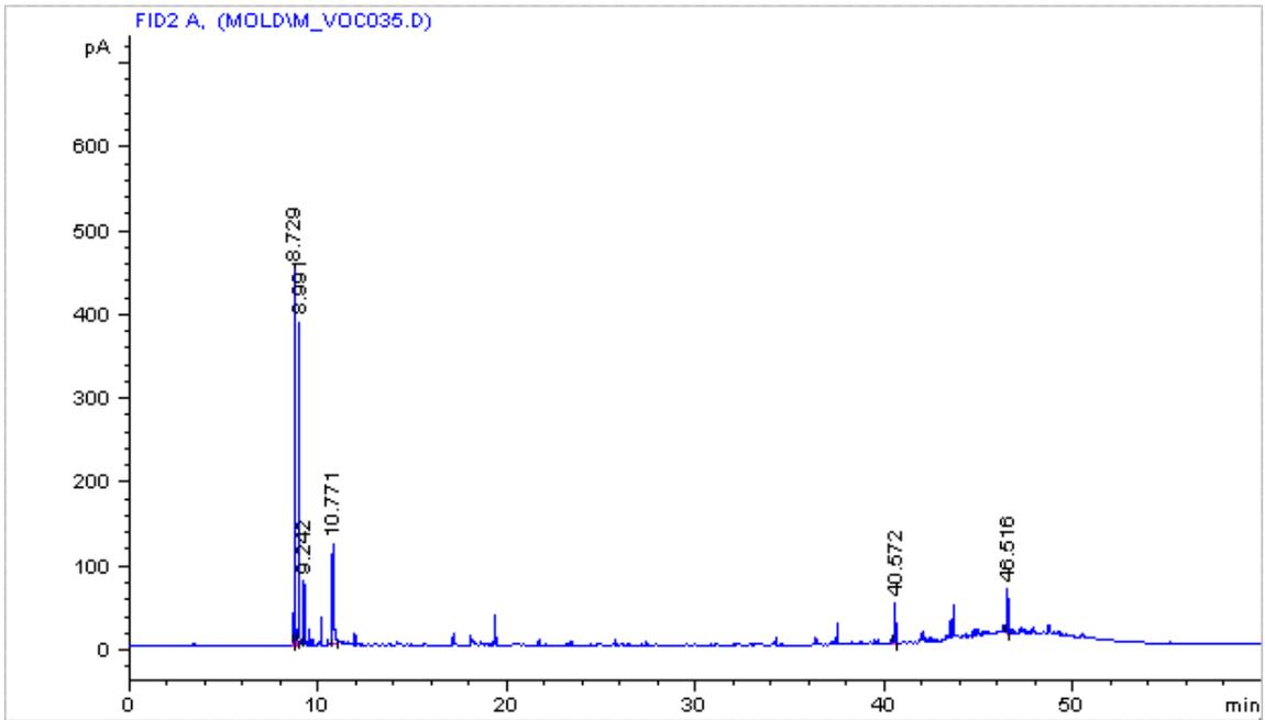
**Figure 17** Chromatogram for the back sample tube collected from purge air flowing at 15 ml/min over *Penicillium* growing on a dusty fiberglass filter for 4 hours on 4/26/99.
