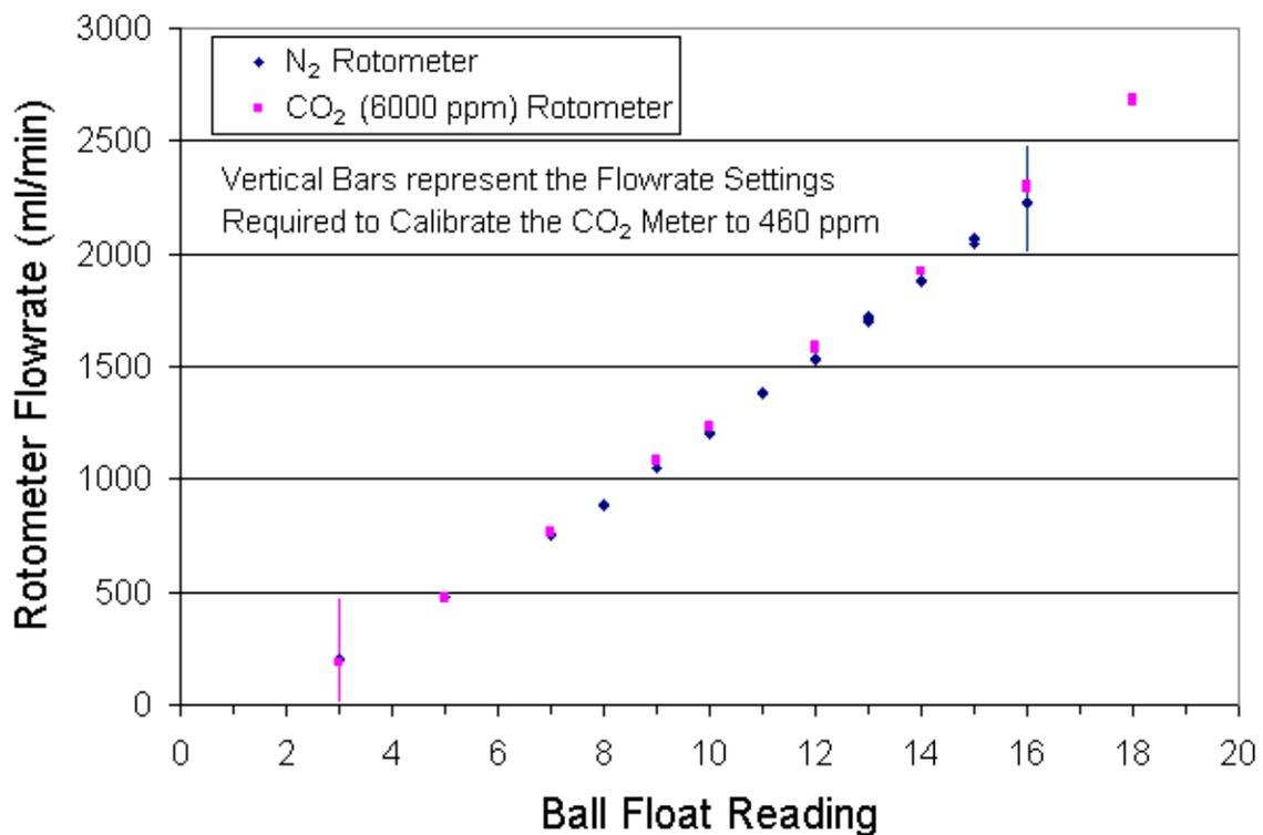
**Figure 29** Flowrate chart for the two rotometers used to calibrate the LicorCO<sub>2</sub> meters.
