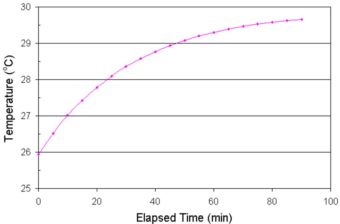
**Figure 26** False temperature readings due to the heat from the instrument. Increasing 3.5°C over the first hour and a half of operation.
