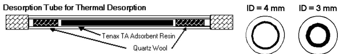
**Figure 7** Profile and cross section views of the thermal desorption tubes used for sampling VOCs.
