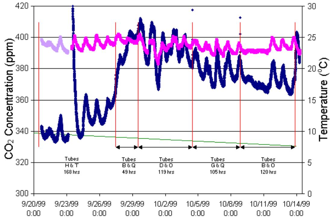
**Figure 37** *Aspergillus* on fiberglass filter #3 for GCMS. Temperature in pink and CO<sub>2</sub> concentration in dark blue. Airflow = 14 ml/min. Tubes D and G sent to Dr. Wang for GCMS analysis. Interpolation of pre and post air tank readings in green.
