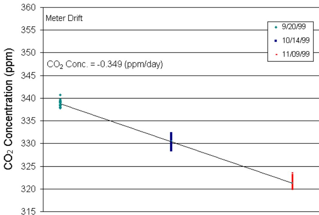
**Figure 31** Three air tank readings showing the drift of the CO<sub>2</sub> meter.
