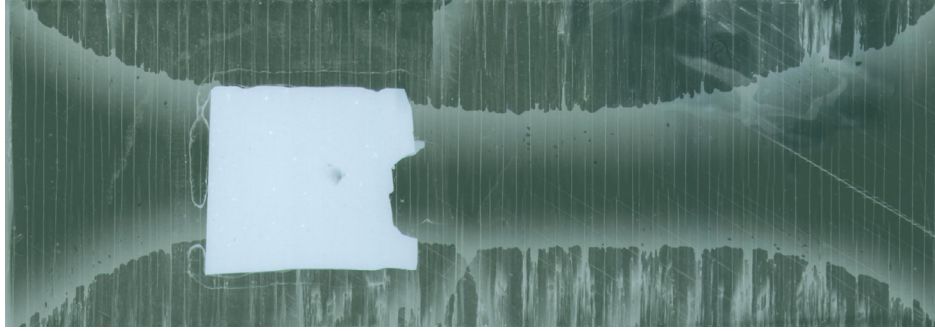
Figure 4.2: A sample radiography shows both transverse matrix cracking and areas of edge delamination.
