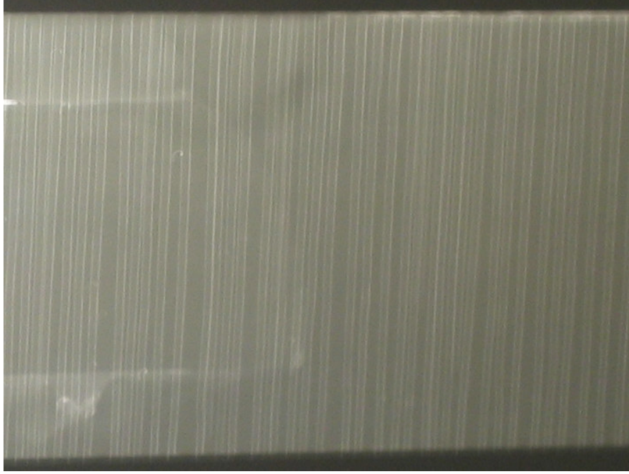
Figure 3.4. An enlarged X-ray shows the cracks for a portion of one of the samples. The total number of cracks are counted to get a value of cracks per centimeter.
