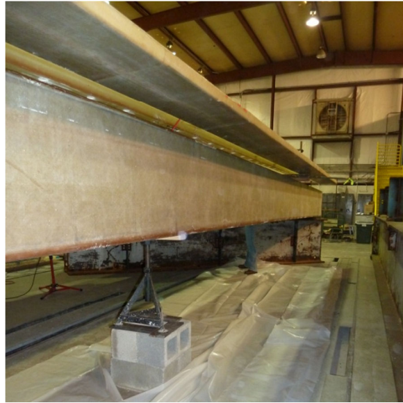
Figure 4-2 Screwjack Introducing Camber into HCB
