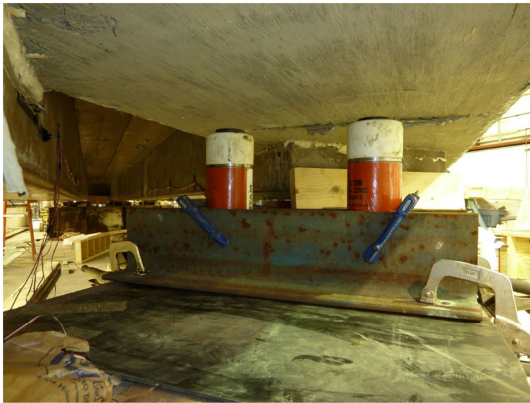
Figure 4-27 Actuators Placed under Diaphragm
