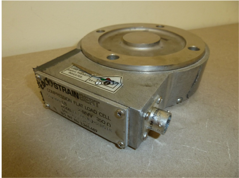
Figure 3-28 50 Kip Load Cell used for Phase II
