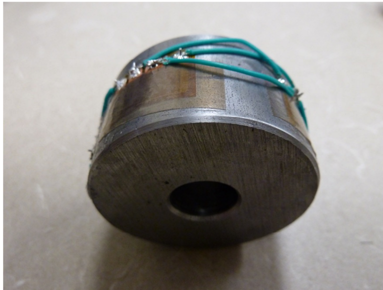
Figure 3-31 Support Load Cell Construction
