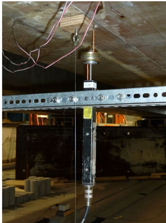
Figure 3-32 LVDT Mounted on HCB 1 at Midspan
