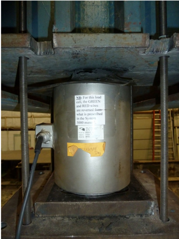
Figure 3-29 300 Kip Load Cell used for Phase III
