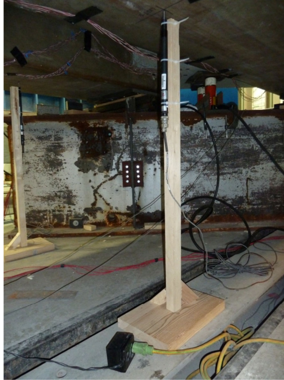
Figure 3-34 LVDT Mounted to Mobile Support
