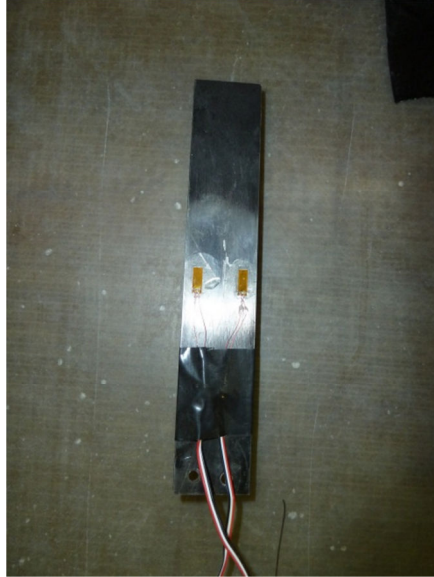
Figure 4-15 Clicker used to Synchronize Data Systems
