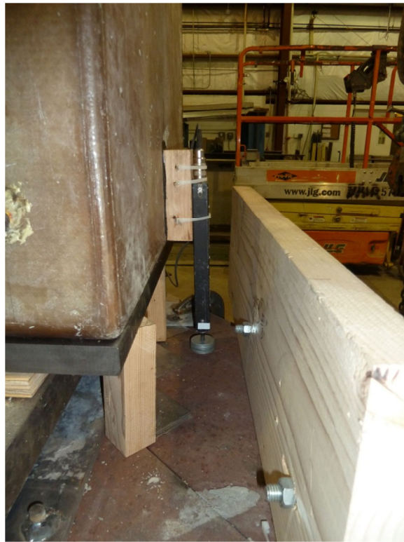
Figure 3-33 LVDT Mounted at Acute Corner
