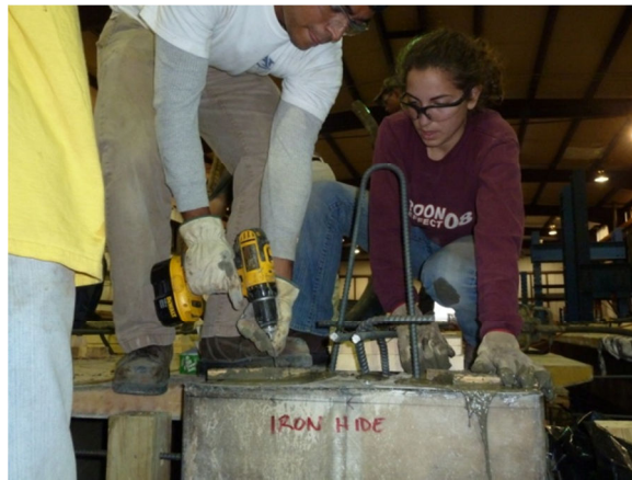
Figure 4-13 Plywood Caps Sealed at HCB End
