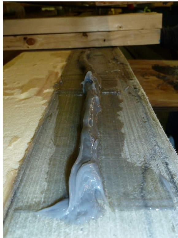
Figure 4-3 Epoxy used to Glue FRP Lid
