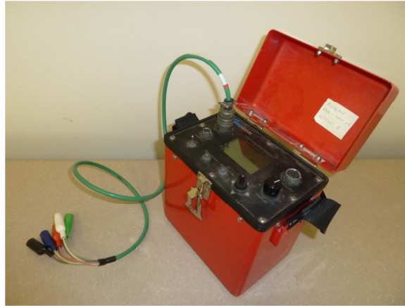
Figure 3-20 Geokon Readout Box
