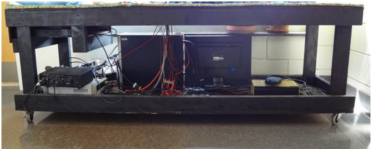
Figure 4.4: Photo of the custom built test bed used to house components and transport the simulator.
