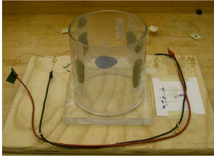
Fig. 5.3 Test stand one; 15 cm diameter lexan cylinder.
