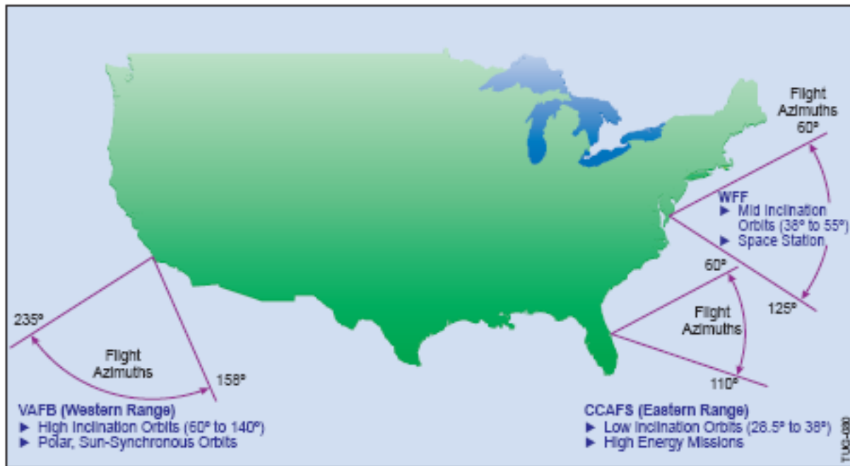
Figure 3.3: Possible Inclination Angles from Various USA Launch Points [7]
