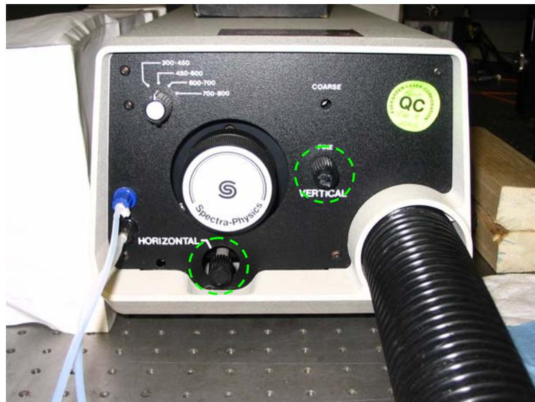
**Figure A-1.** Laser head rear panel showing vertical and horizontal rear reflector controls.
