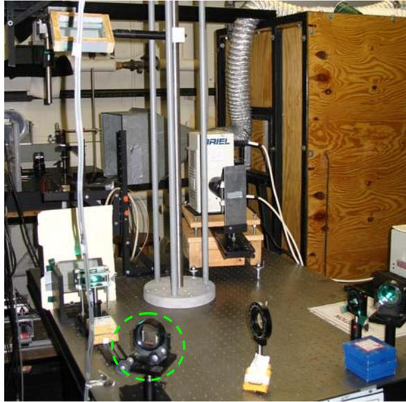
**Figure A-4.** Image showing third beam mirror location.
