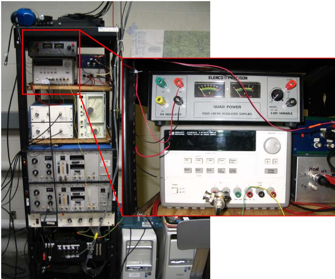
**Figure E-3.** Electronic pressure regulator power supply and control voltage source.
