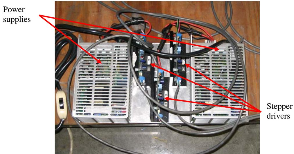
**Figure F-3.** Three stepper drivers mounted together (center) along with their power supplies (outside).
