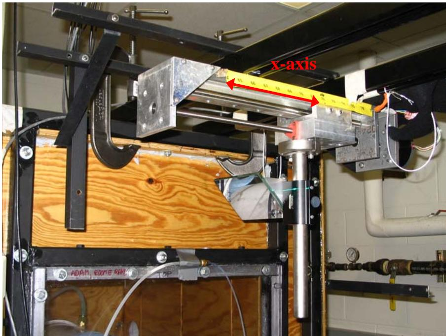
**Figure F-1.** Single translation stage used for Mie scattering flow visualization experiments.
