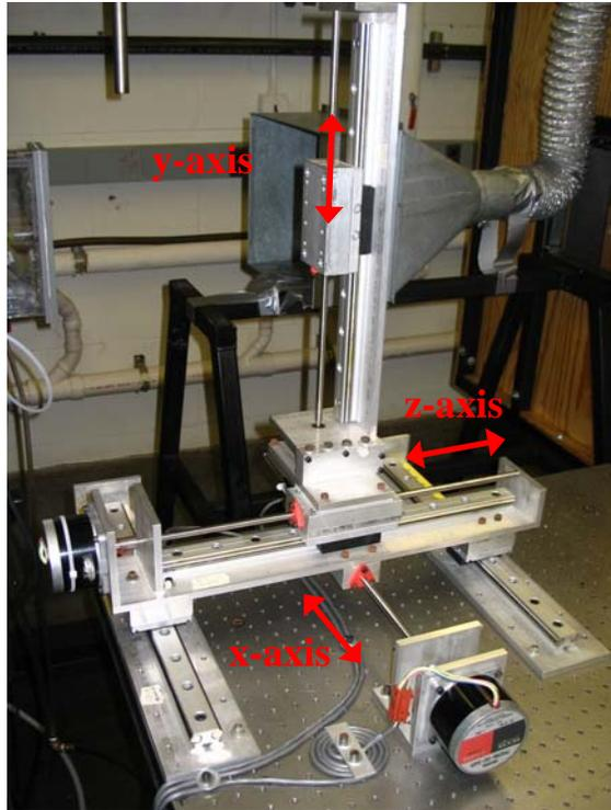
**Figure F-2.** Coupled translation stages providing three axes of motion for the LDV probe.
