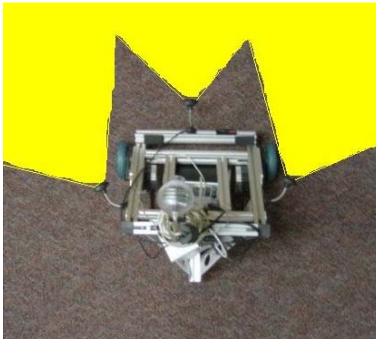
Figure 10: Estimated range of IR sensors. The ER1's back is left blind
